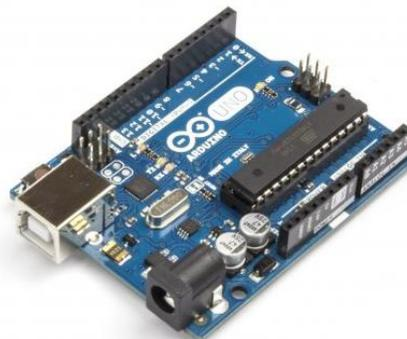
**Figure 133: Arduino Uno microcontroller.**
