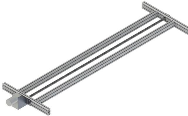
**Figure 104: Vehicle erector track assembly.**
