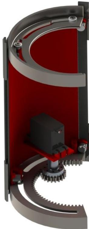
**Figure 44: Complete door and track assembly.**
