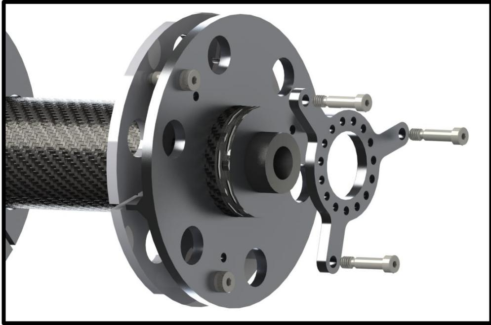
**Figure 15: Motor retention components exploded view.**
