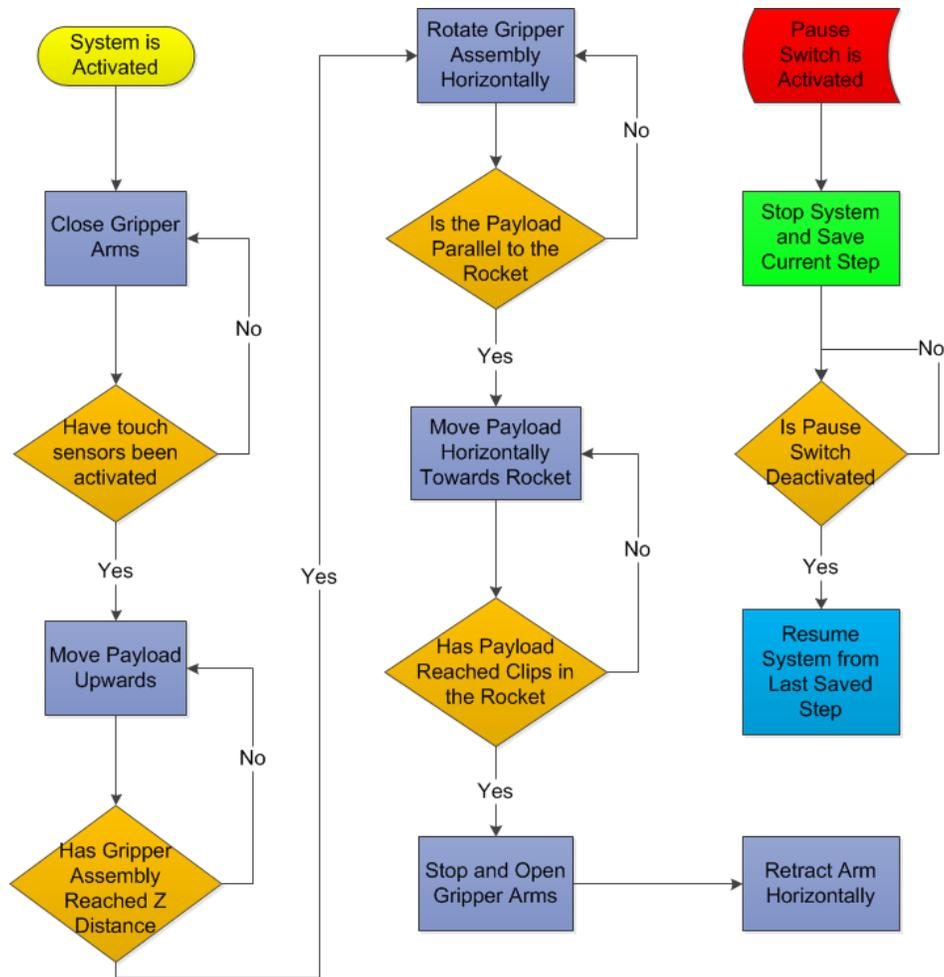
**Figure 71: Flowchart for payload capture system.**
