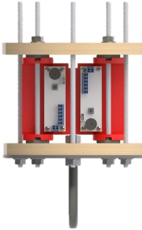
**Figure 29: Altimeter sled full assembly.**
