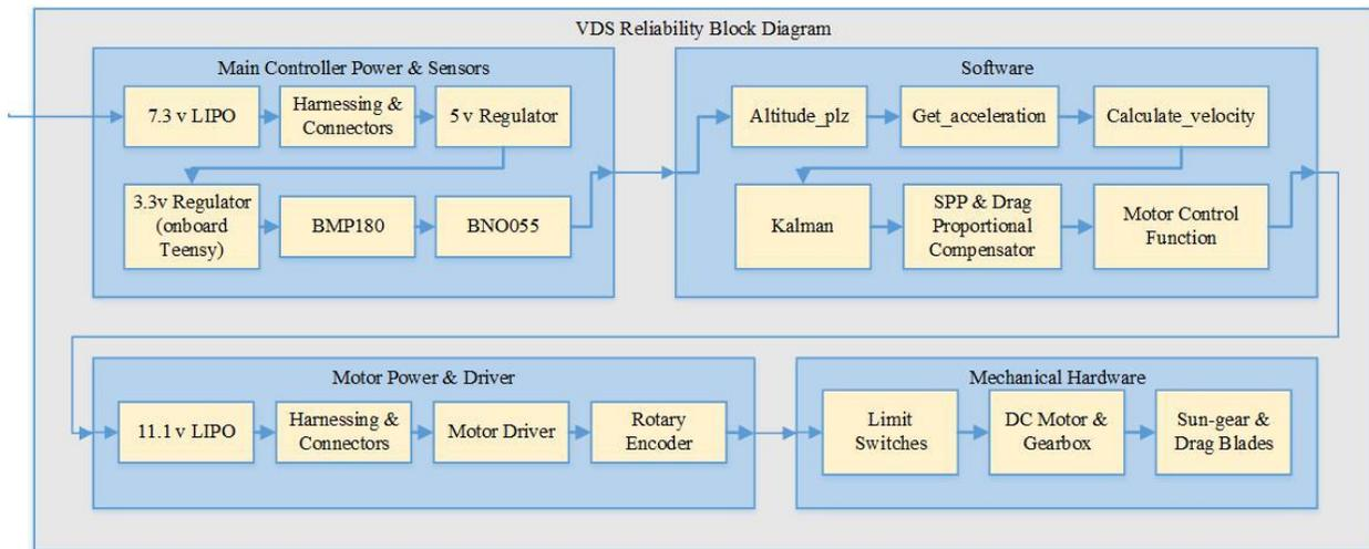
**Figure 91: Reliability block diagram for VDS.**
