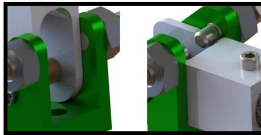
**Figure 112: Detailed view of the Lock Pin being restrained in the stowed configuration (Left) and being engaged into the lock pin contour feature in the Arm Pivot (Right).**
