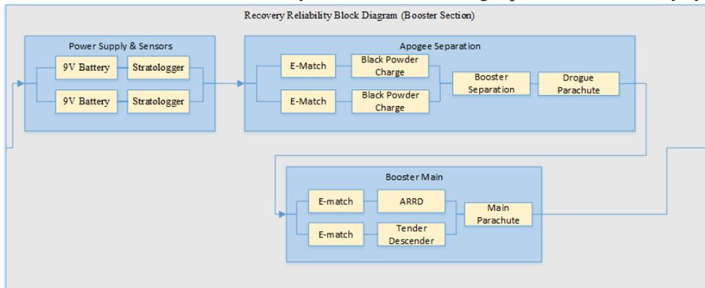
**Figure 89: Reliability block diagram for booster section.**
