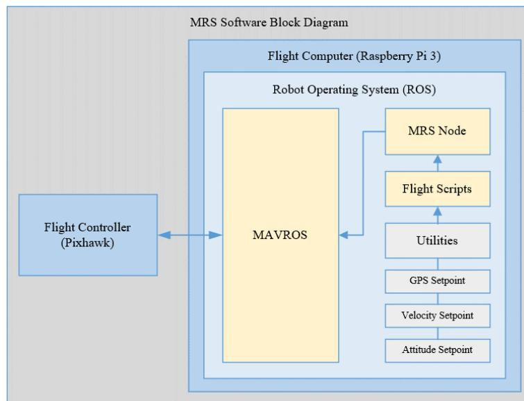
Figure 104: Block diagram of the MRS software.
