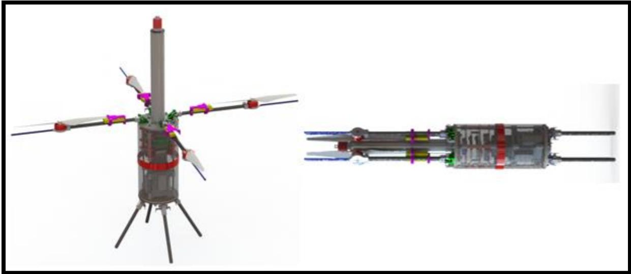
Figure 101: Rendering of the Experimental Payload (left; deployed, right; stowed).
