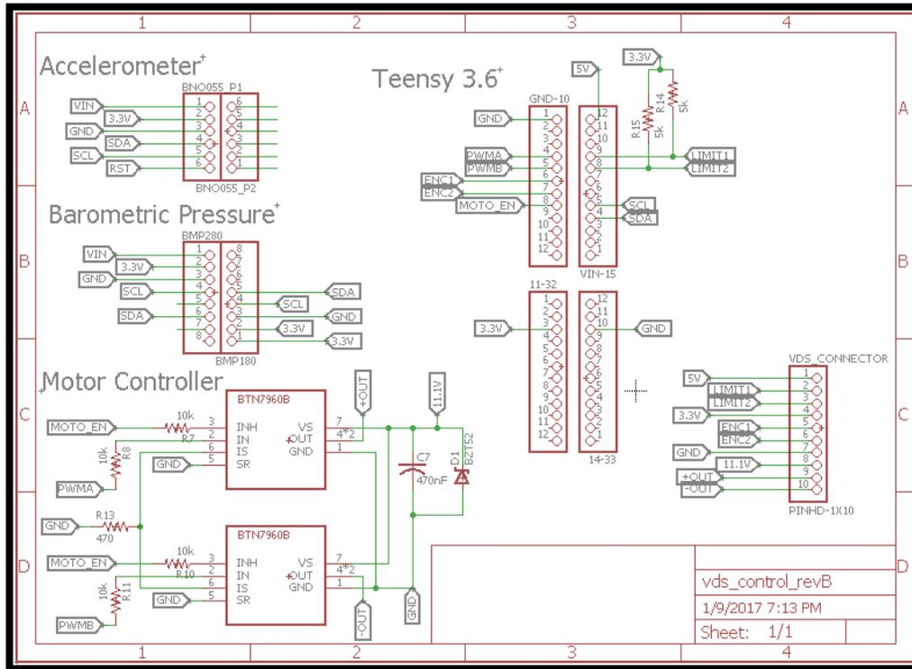
Figure 6: System control board revision B
