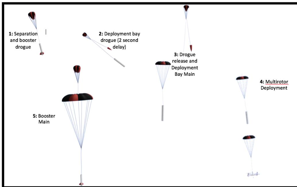
Figure 57: Illustration of recovery sequence.
