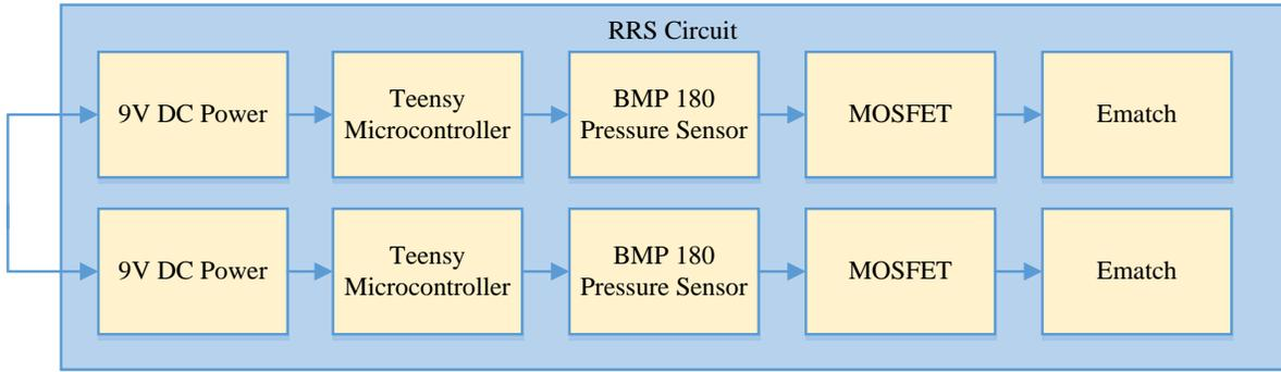
**Figure 93: Reliability block diagram for RRS circuit.**
