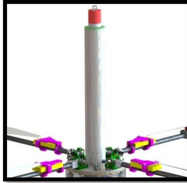
**Figure 123: Rendering of the RRS mechanism.**
