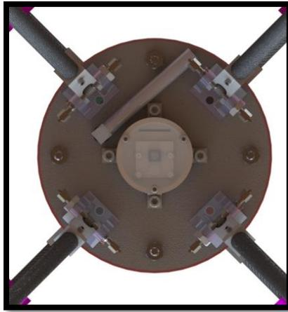
**Figure 126: TDS Camera housing mounted onto Lower Bulkplate Assembly.**
