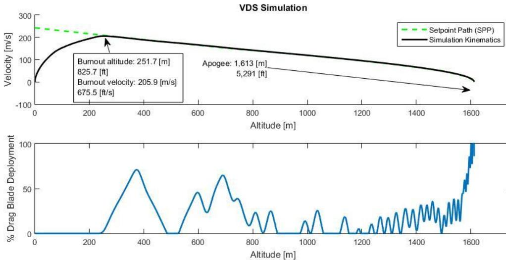
Figure 75: VDS simulation of full scale vehicle.
