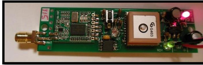
**Figure 39: Eggfinder GPS tracking device.**
