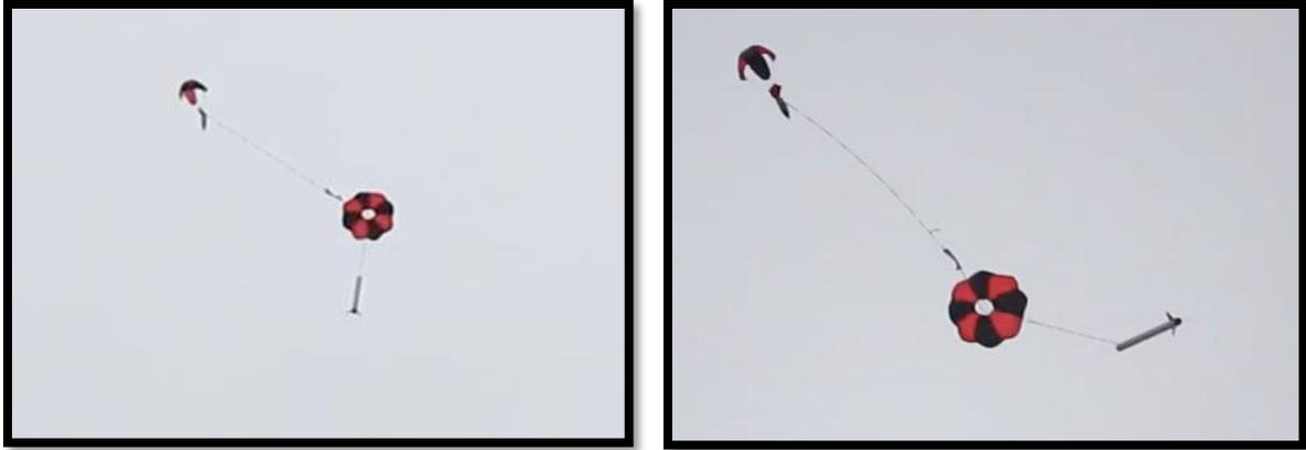
**Figure 53: Severe instability caused by drogue and nosecone**
