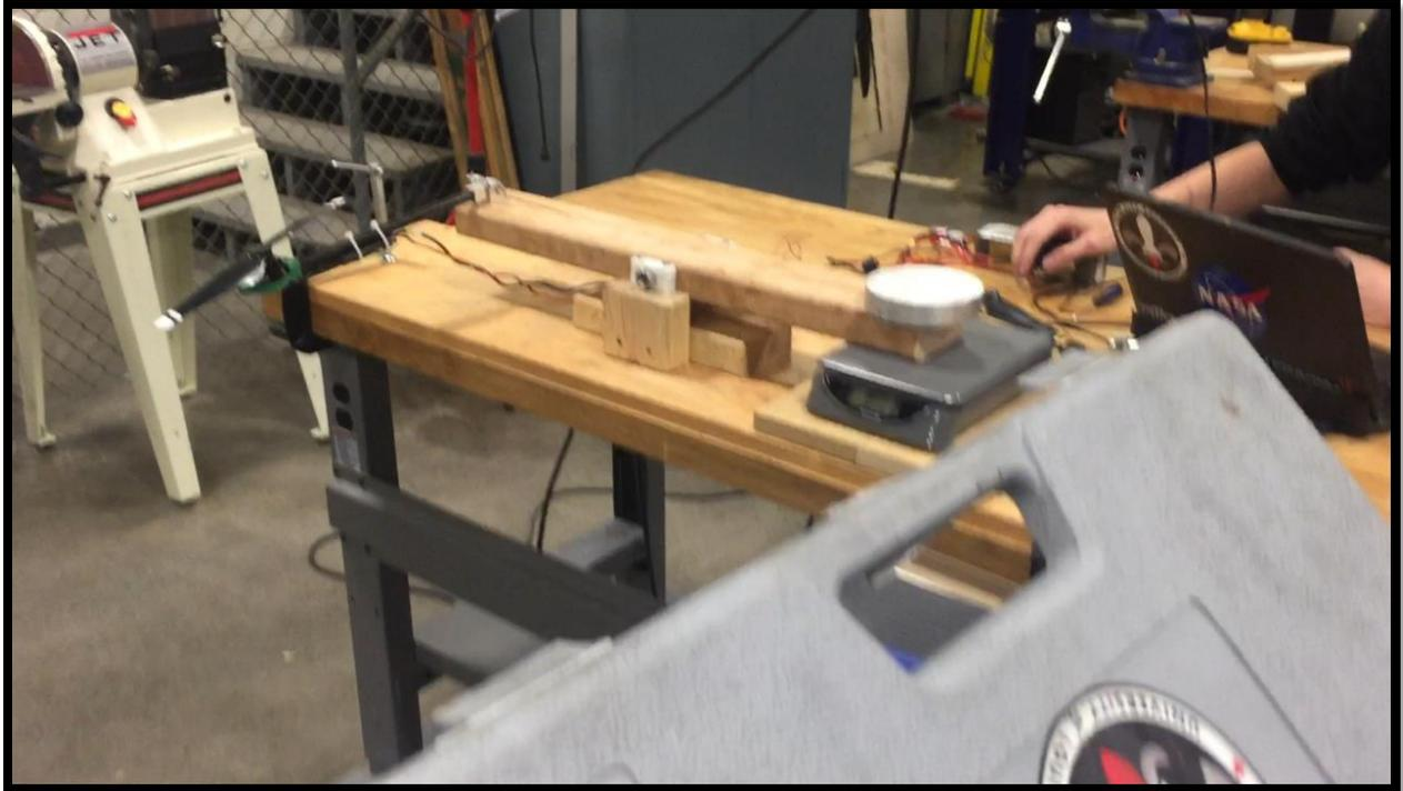
**Figure 142: See-Saw Pivot Test Rig with Propulsion Arm**
