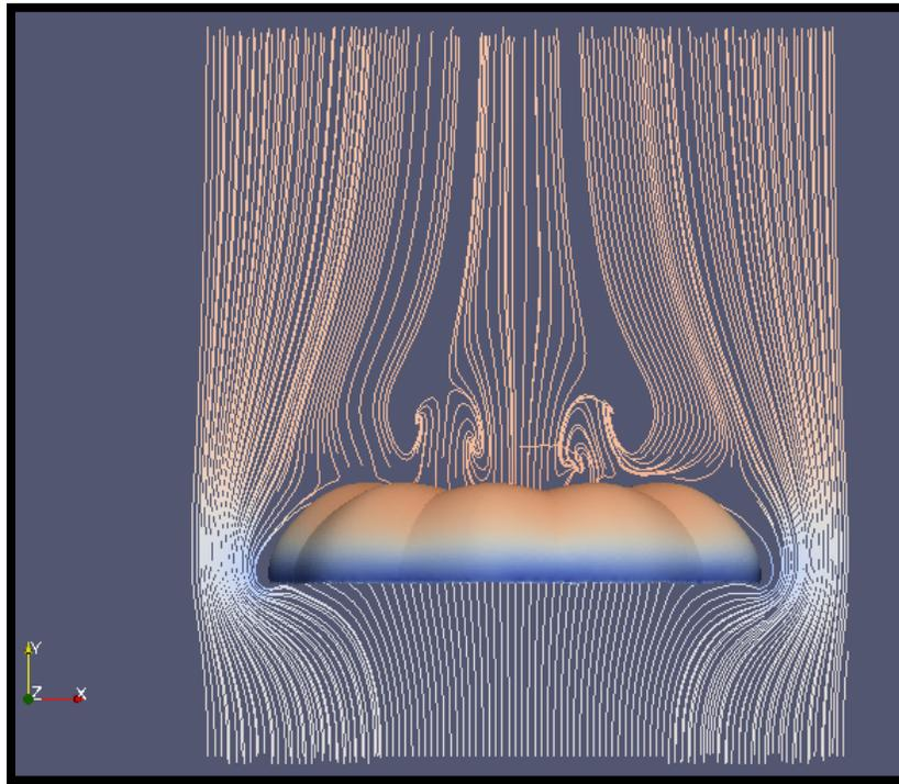
**Figure 61: Drag profile of toroidal parachute.**
