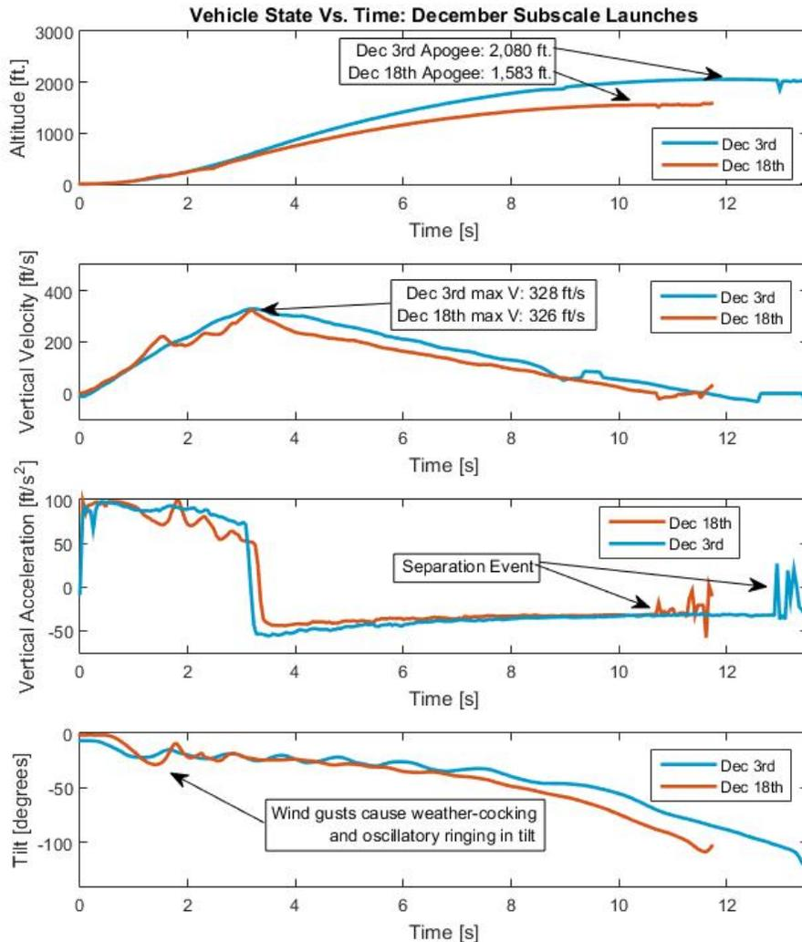
**Figure 43: Vehicle State Vs. Time: December subscale launches.**
