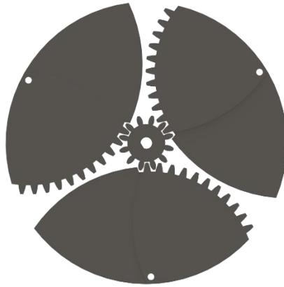
**Figure 16: Gear Meshing of Drag Blades.**
