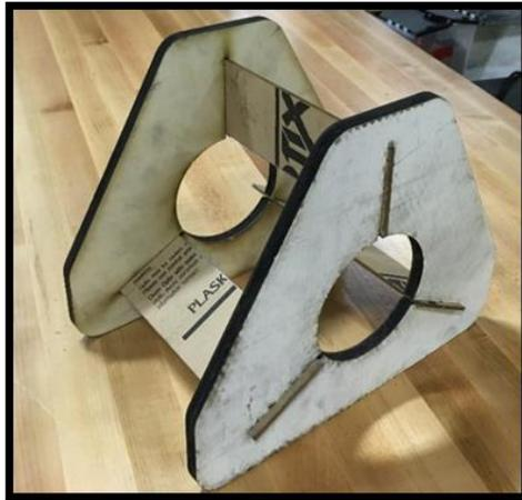
Figure 26: Fin slot alignment jig.
