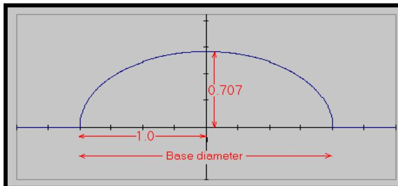
**Figure 62: Ellipsoid parachute side profile**
