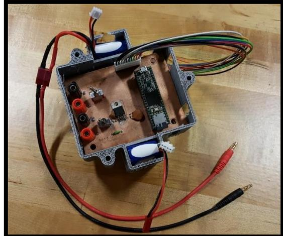
**Figure 13: VDS electronics PCB prototype and sled.**
