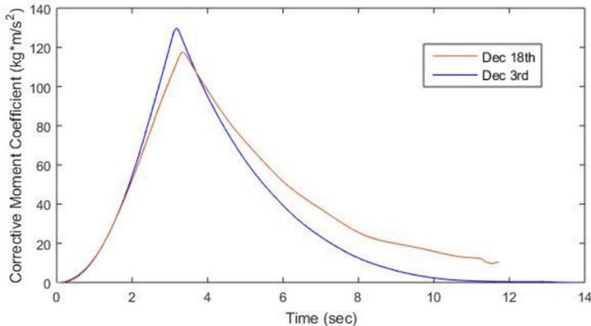
**Figure 48: Corrective Moment Coefficient of the subscale vehicle for each launch.**
