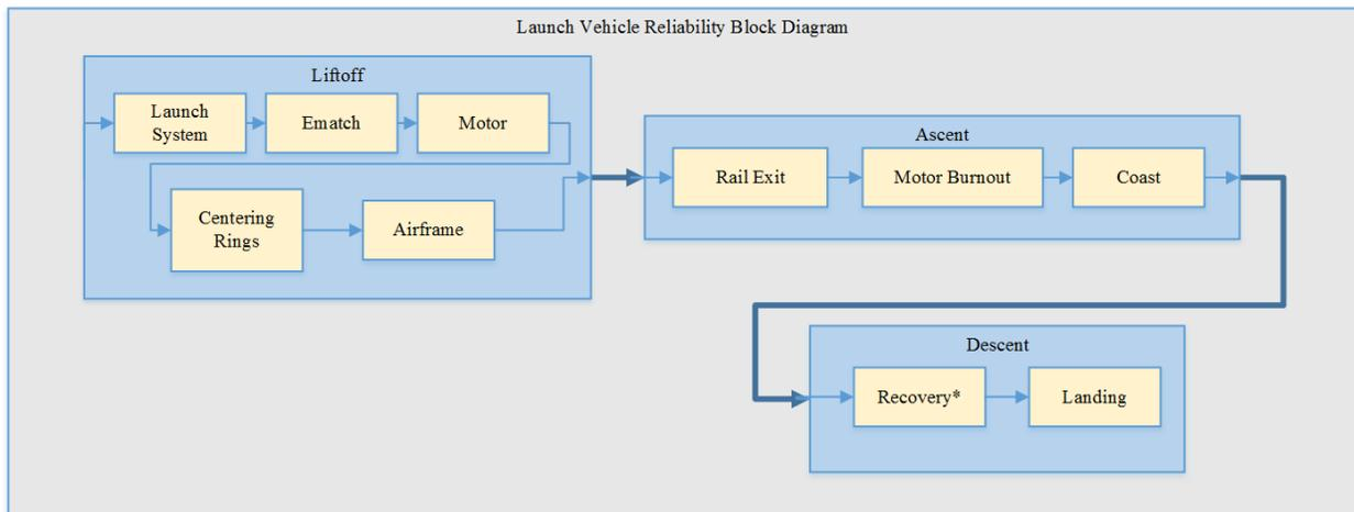
**Figure 86: Launch vehicle reliability block diagram.**
