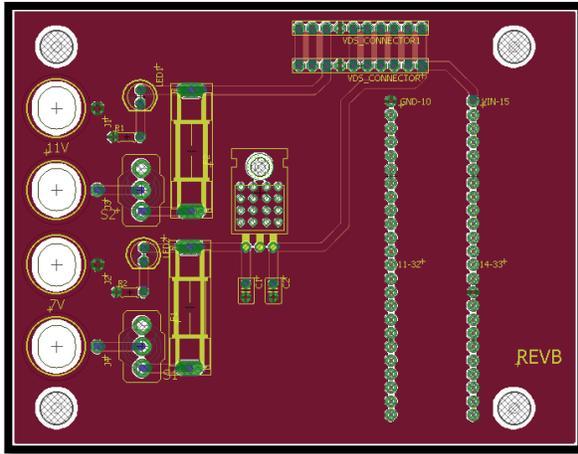
**Figure 10: Power distribution board revision B.**
