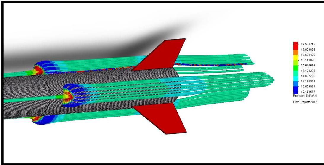
**Figure 68: VDS air flow CFD simulation results.**
