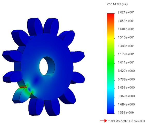
**Figure 23: Central gear teeth FEA stress plot.**
