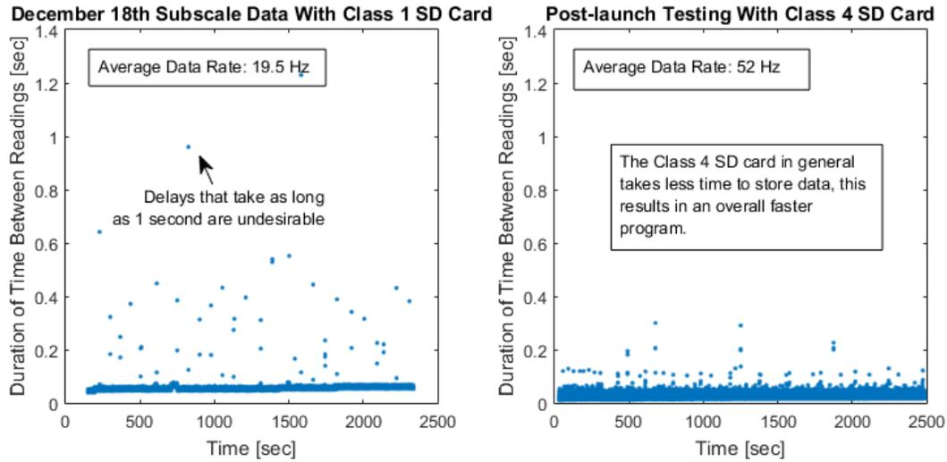
**Figure 140: Visualization of delays in VDS Test Electronics software.**
