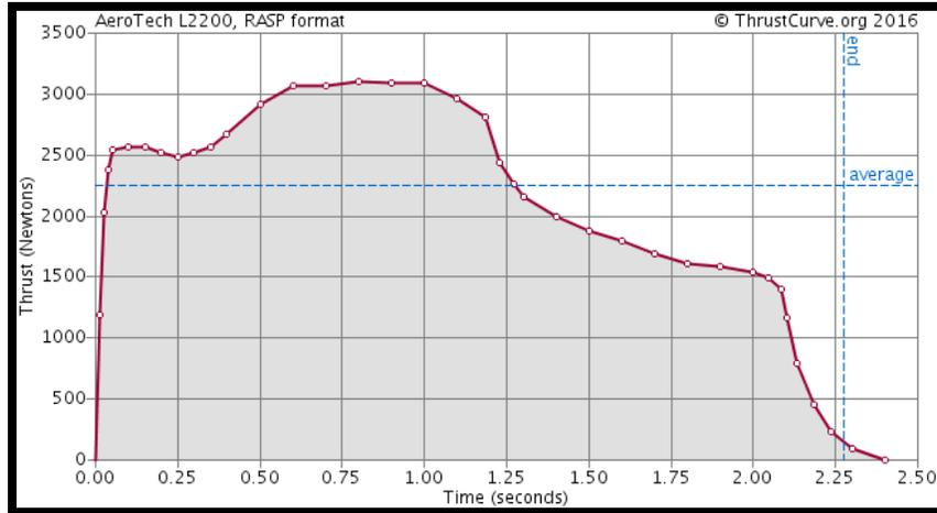
**Figure 84: Aerotech 2200G Thrust Curve.**
