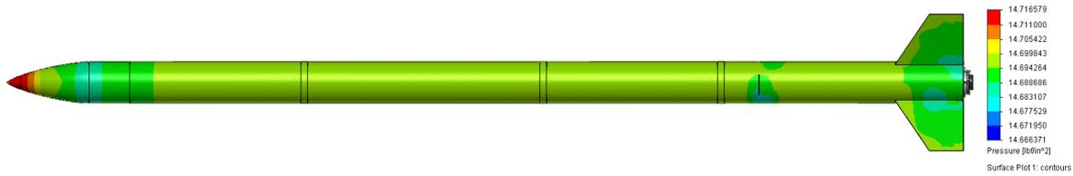
**Figure 79: CFD simulation surface pressure results.**
