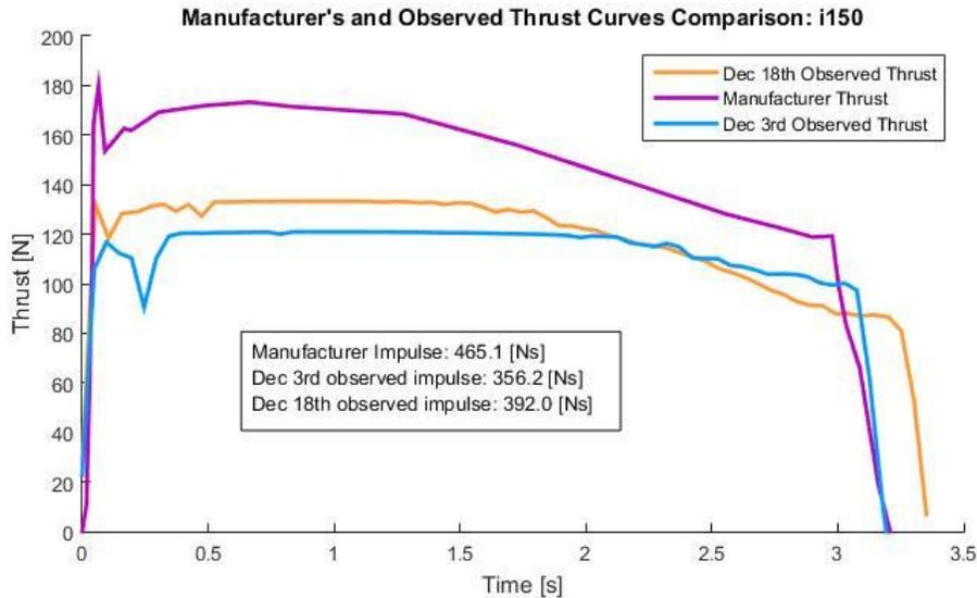
**Figure 55: Observed and Manufacturer's thrust curves for I150 motor: December 18<sup>th</sup> subscale.**
