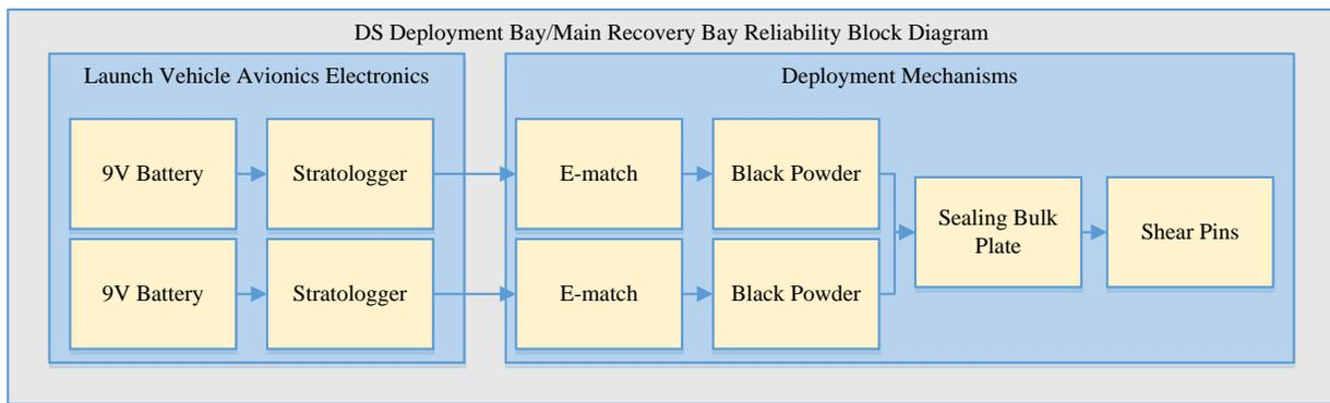
Figure 96: Reliability block diagram for DS.
