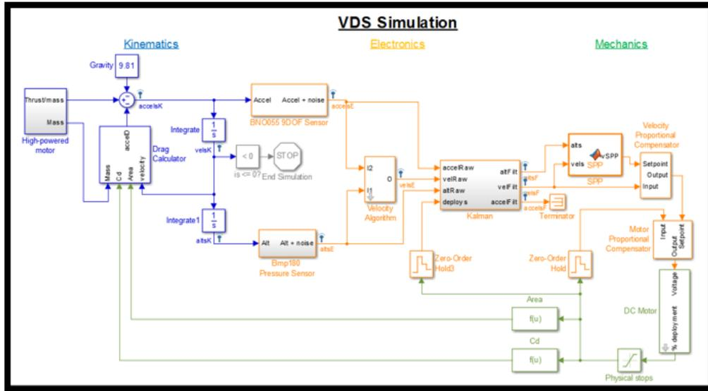
Figure 74: VDS simulation Simulink blocks.
