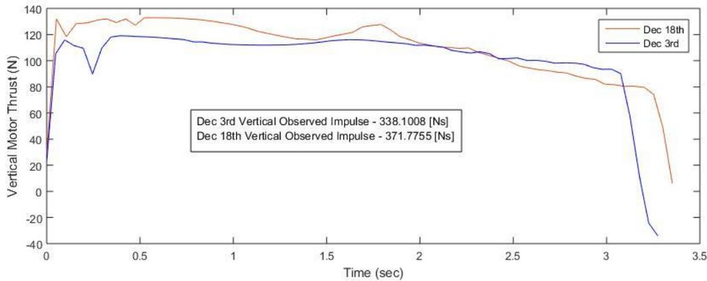
**Figure 50: Observed vertical motor thrust of the Cesaroni I150 for both subscale launch.**
