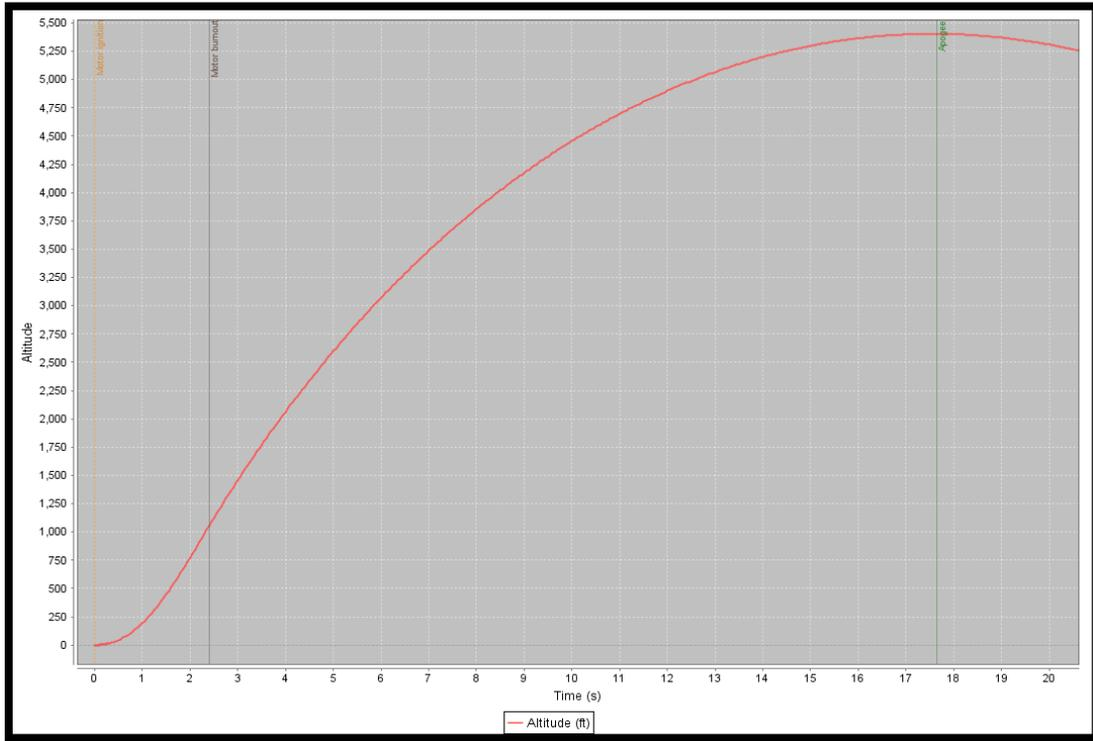
Figure 70: Altitude vs time without VDS.
