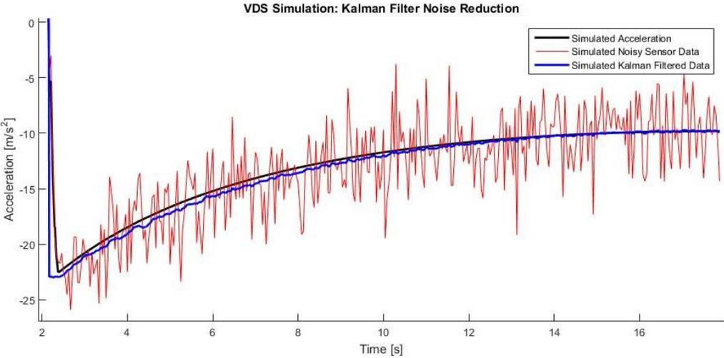
Figure 77: VDS simulation Kalman Filter noise reduction example.
