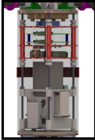
**Figure 129: Coupler body with all thread mounting rods.**
