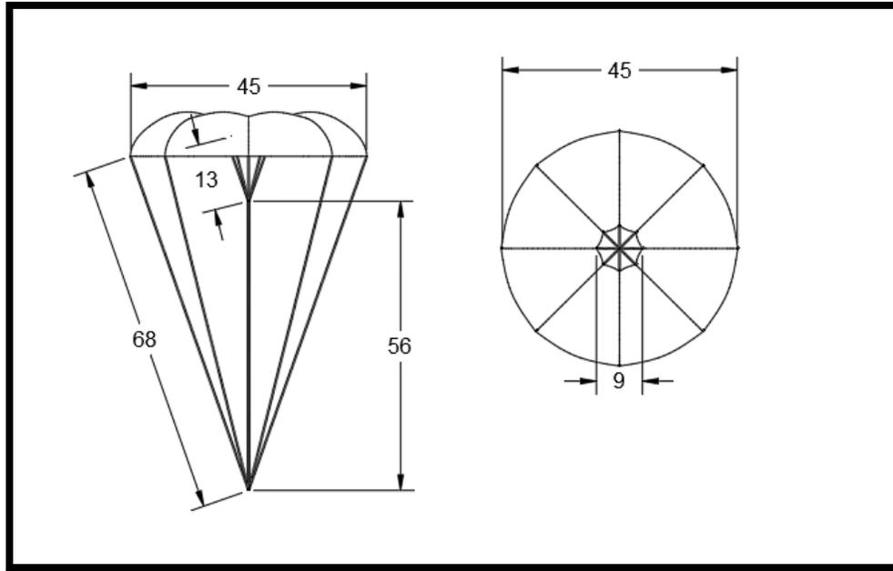
**Figure 64: Dimensions of deployment bay main**
