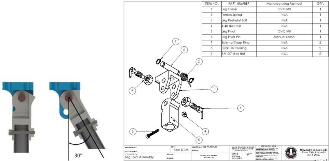
Figure 135: LLS stowed and deployed configuration with deployment angle and Detailed drawing of the Leg Pivot Assembly.
