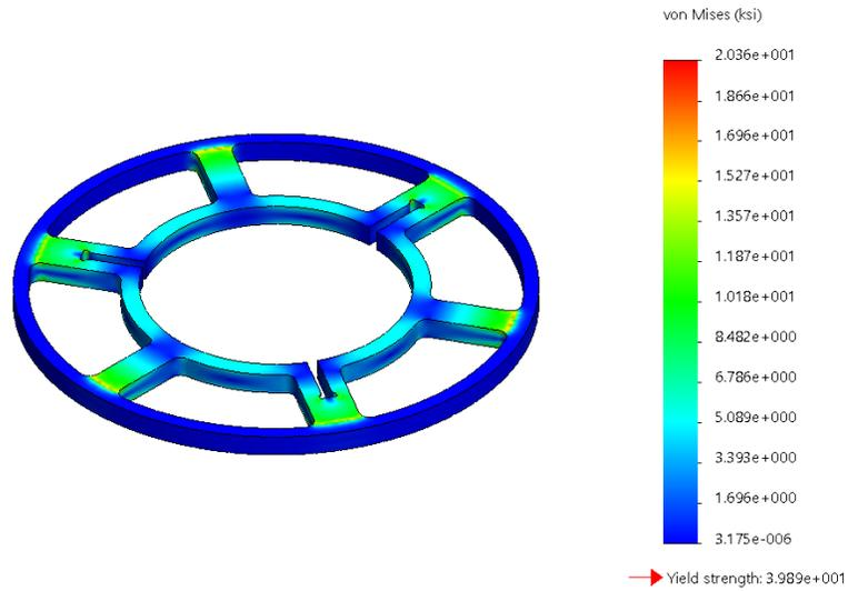
**Figure 31: Finite element analysis stress plot.**
