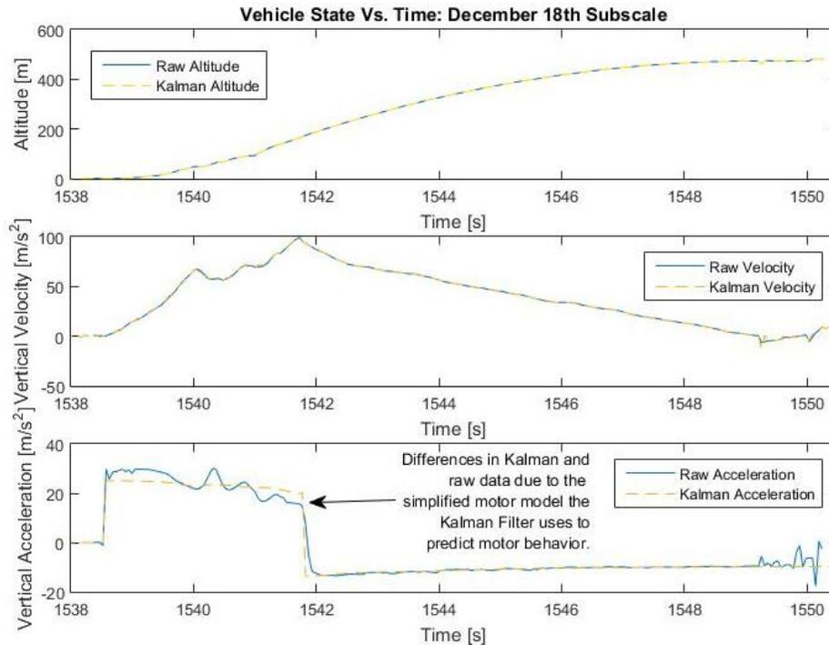
**Figure 141: Kalman filtered and raw state signals.**
