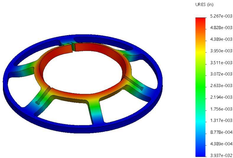
**Figure 32: Finite element analysis displacement plot.**
