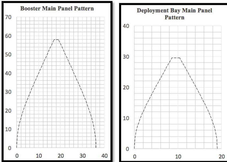
**Figure 65: Main parachute panel geometries. Axes in inches. (Note: Not to scale)**
