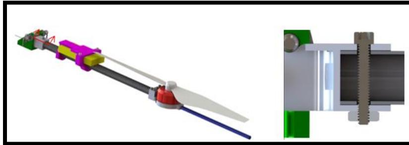
**Figure 111: Detailed section view of the interaction between the Arm Pivot, Restraint bolt, Jam nut, and Carbon Fiber Arm.**
