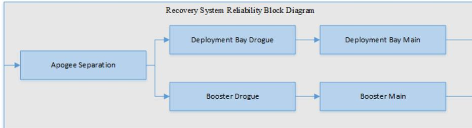
**Figure 88: Reliability block diagram showing overview of recovery system.**
