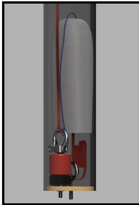
**Figure 42: Subscale recovery layout**
