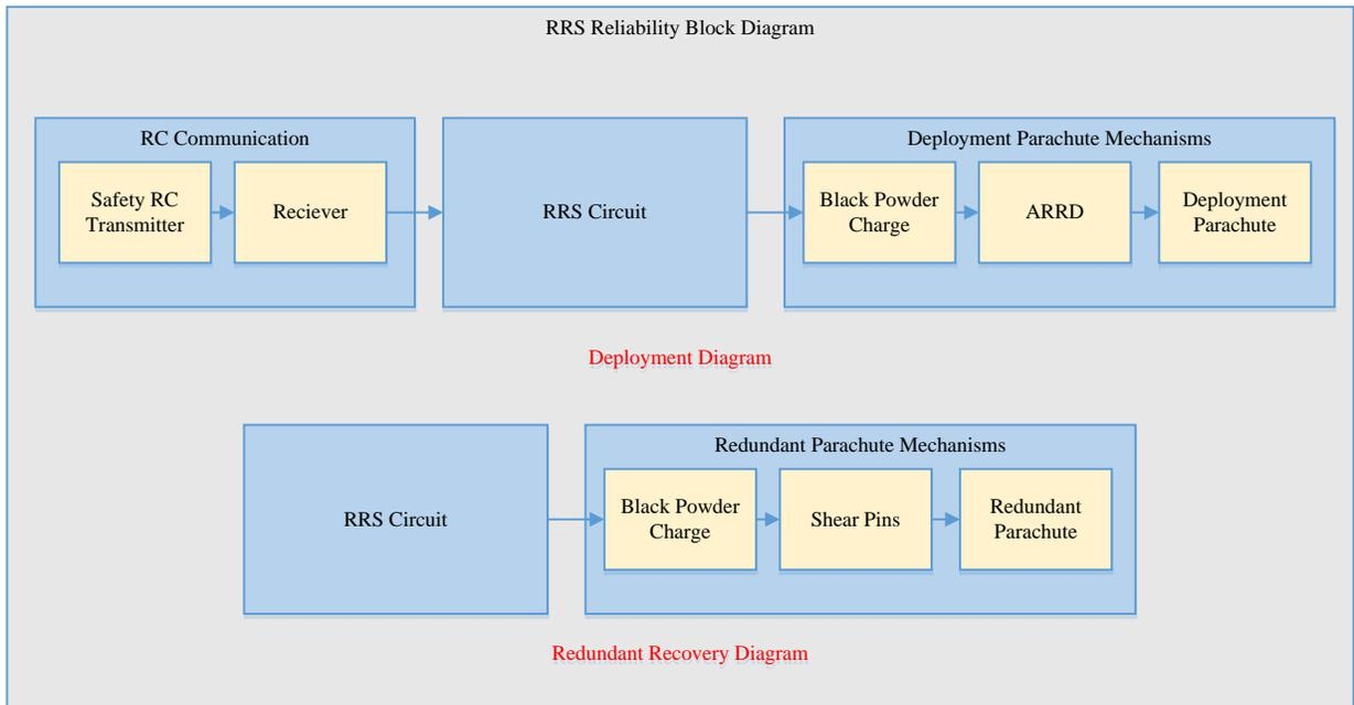
**Figure 94: Reliability block diagram for the RRS functions.**
