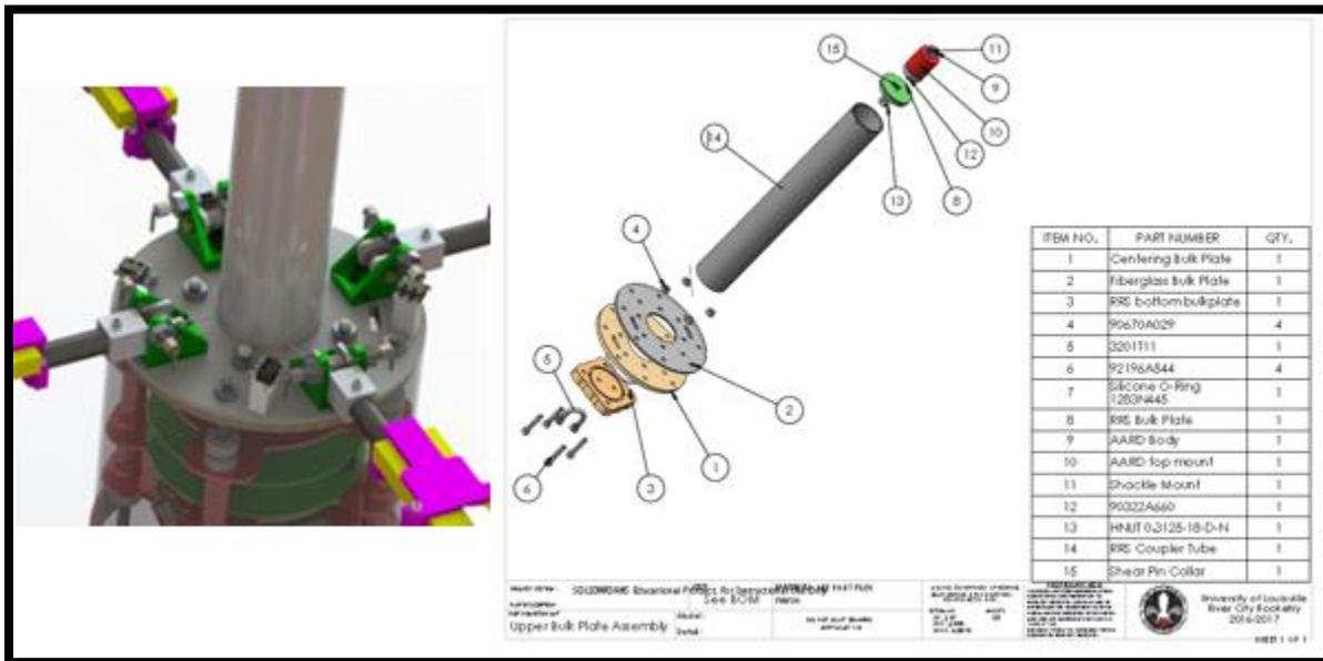
**Figure 128: Rendering and detailed drawing of the Upper Bulk Plate Assembly.**
