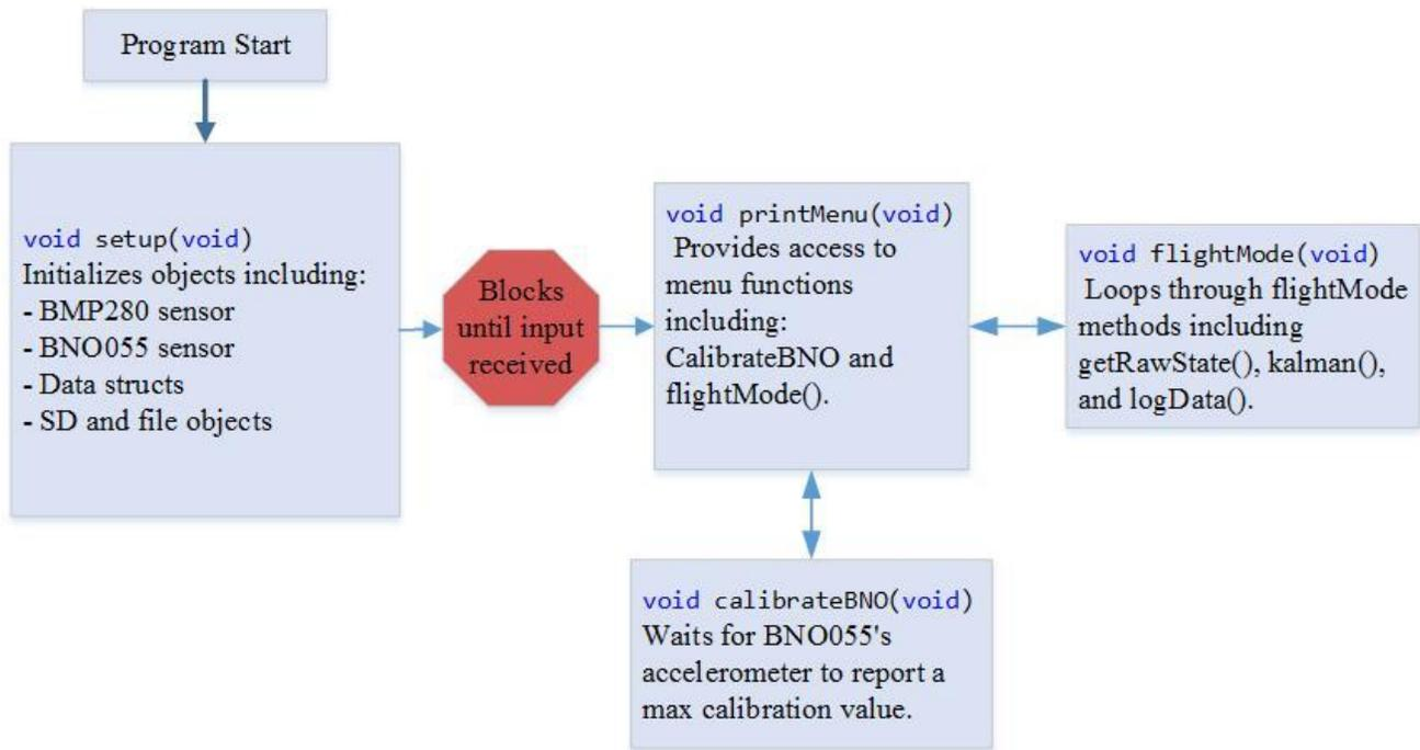
**Figure 4: VDS software functional block diagram.**
