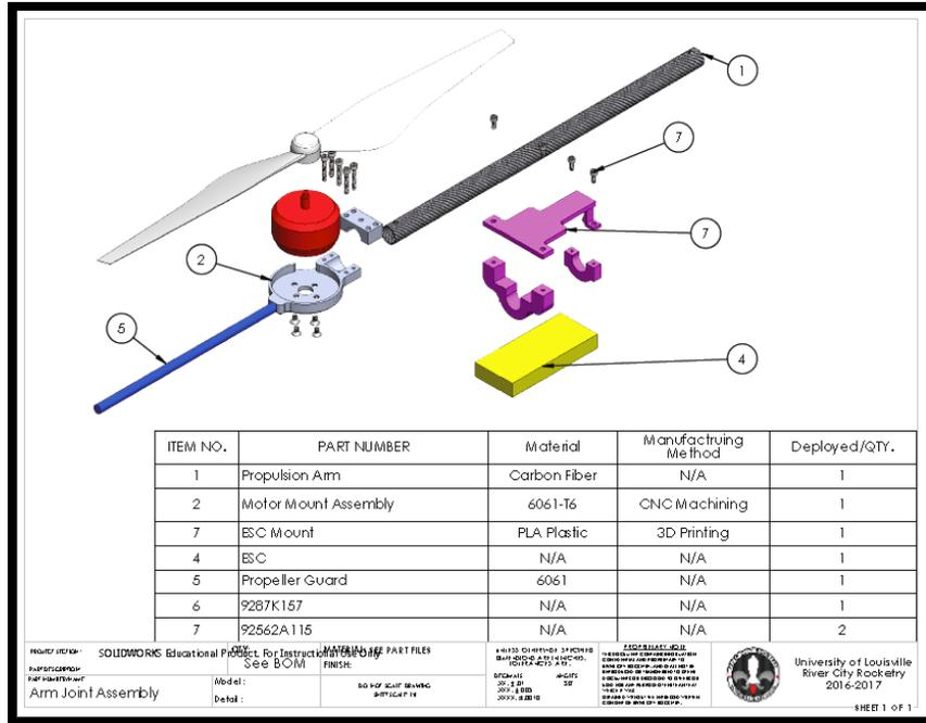
**Figure 115: Detailed drawing and exploded view of the Motor Assembly.**
