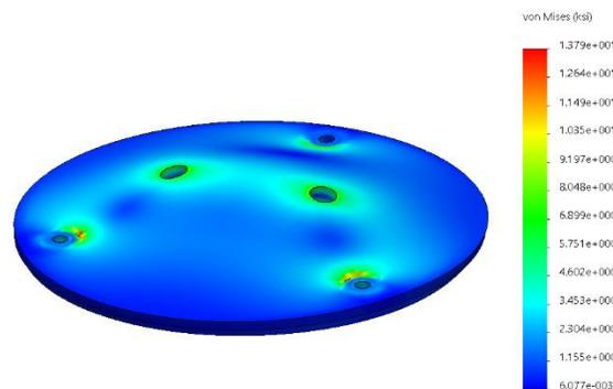
**Figure 38: Bulkplate FEA simulation stress plot.**
