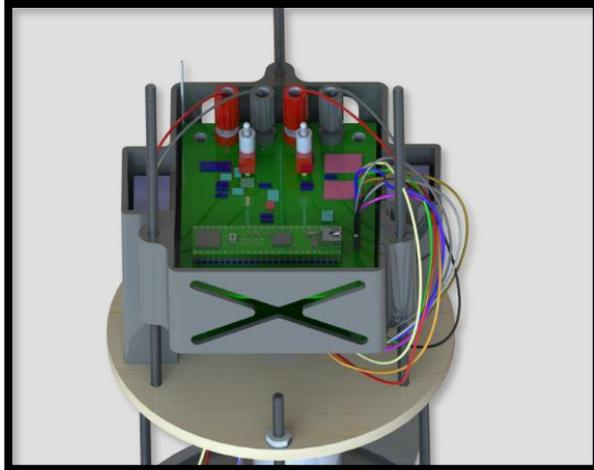
**Figure 12: VDS electronics and sled rendering (attached to bulkplate).**
