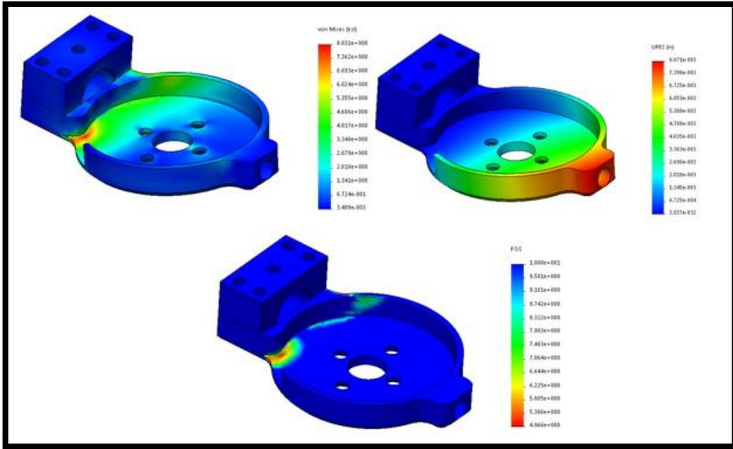
Figure 117: FEA model setup, Von Mises Stress, Deflection, and FOS on the Motor Mount Assembly.
