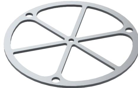
**Figure 21: Rendering of bottom support plate.**
