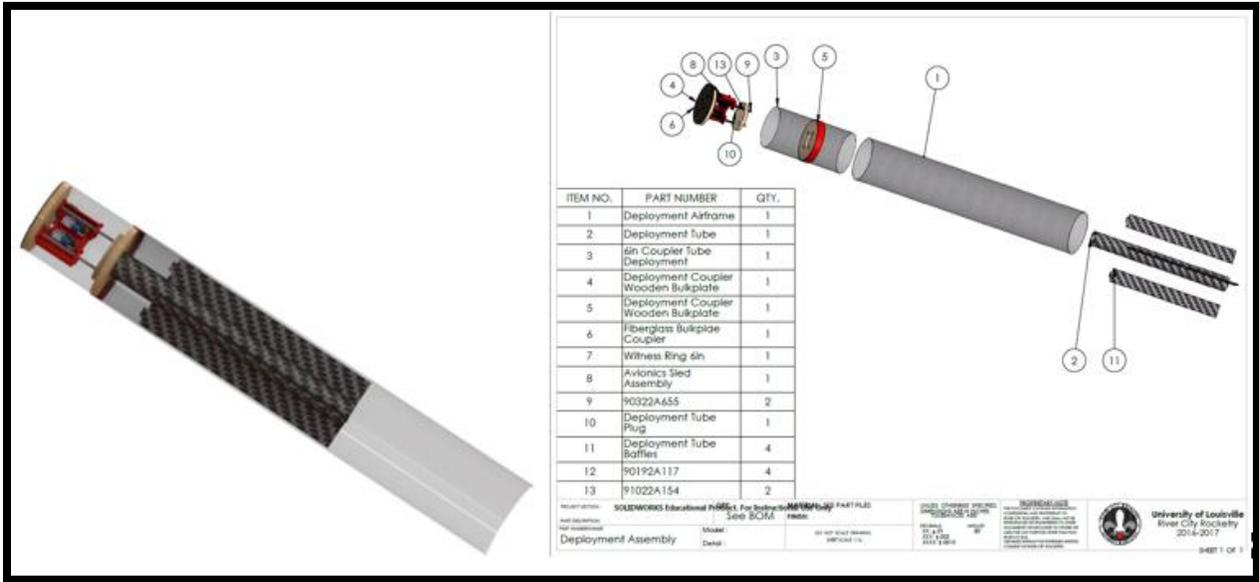
**Figure 136: Deployment Bay section view rendering and detailed exploded view.**
