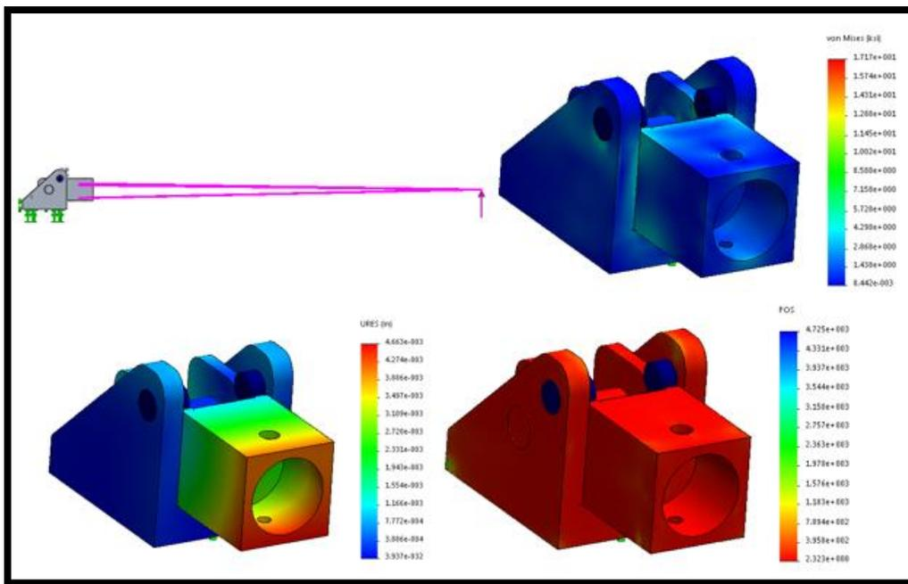
**Figure 116: FEA model setup, Von Mises Stress, Deflection, and FOS on the Arm Pivot Assembly.**
