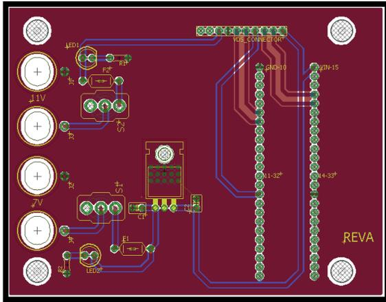
**Figure 8: Power distribution board revision A.**
