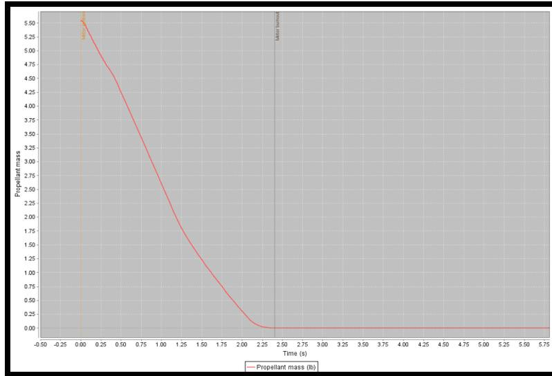
**Figure 72: Propellant mass versus time.**
