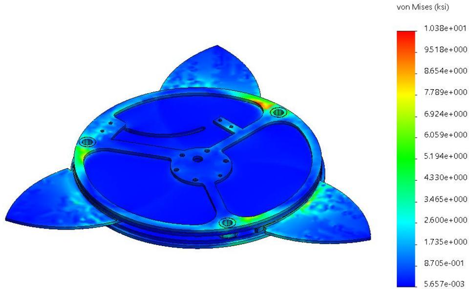
**Figure 24: VDS assembly FEA stress plot.**
