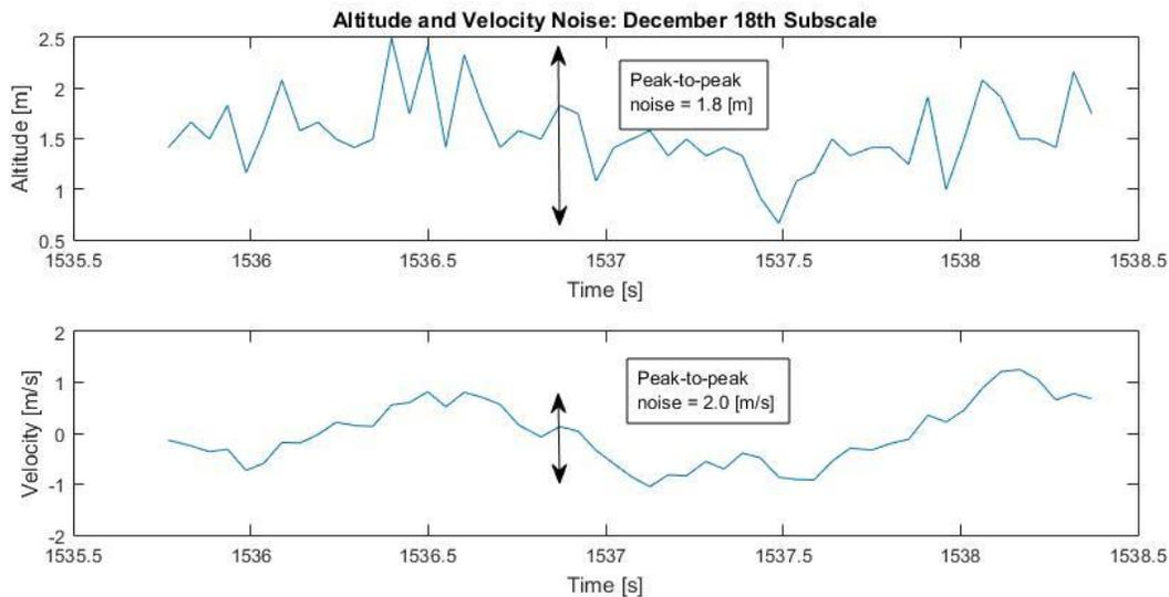
**Figure 139: Altitude and Velocity Noise: December 18<sup>th</sup> Subscale.**
