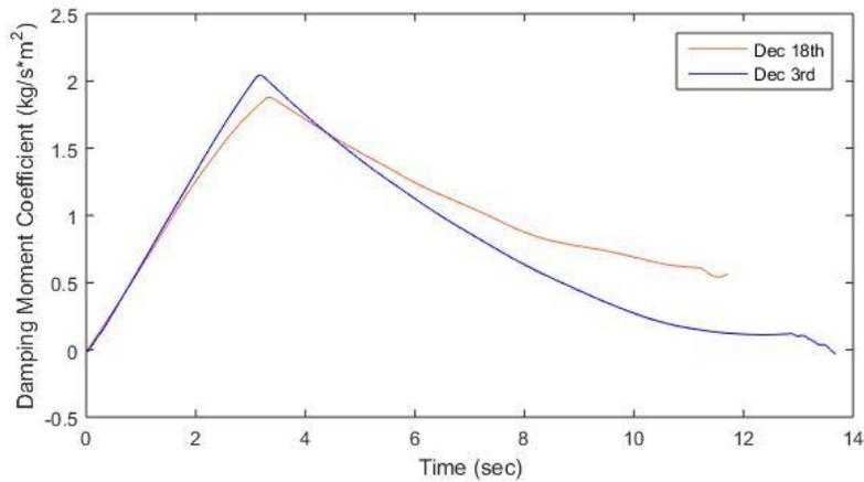
**Figure 47: Damping moment coefficient of the subscale vehicle launches.**
