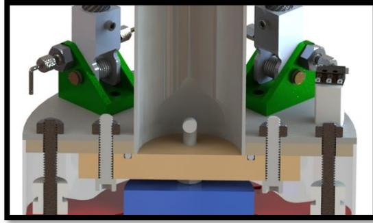
**Figure 125: Section view of the Removable Sealing Bulkplate at the bottom of the RRS Tube.**
