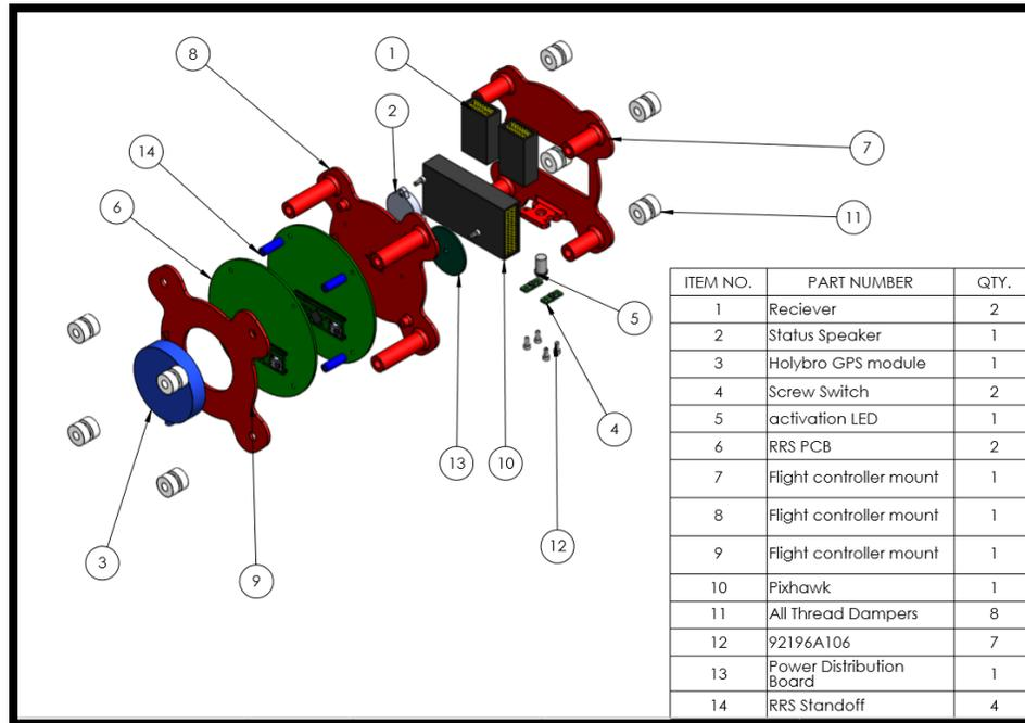
**Figure 131. BOM for all parts, fasteners, and electronics housed in the assembly.**
