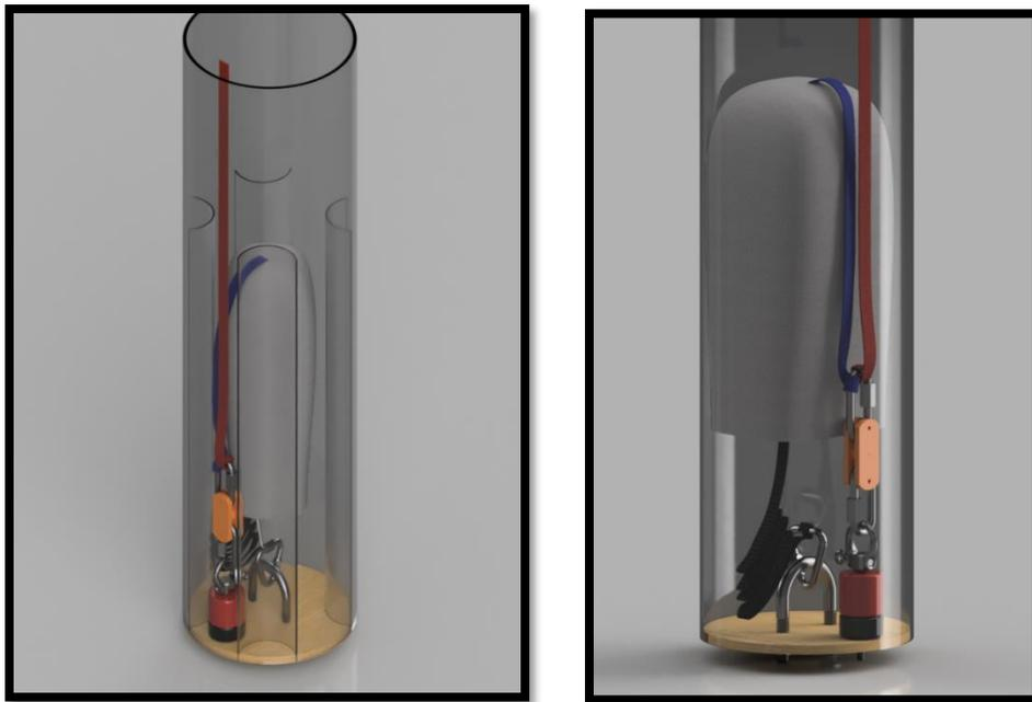
**Figure 58: Transparency of booster recovery layout with payload leg sheaths (left) and deployment bay recovery layout (right) with drogue shock cord (red), deployment bag tether (blue), main shock cord (black), and ARR and tender descender devices.**
