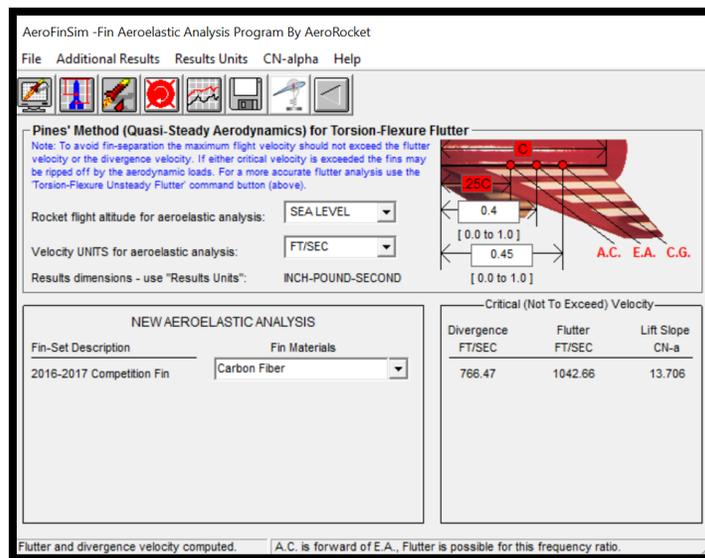
**Figure 81: FinSim simulation results**
