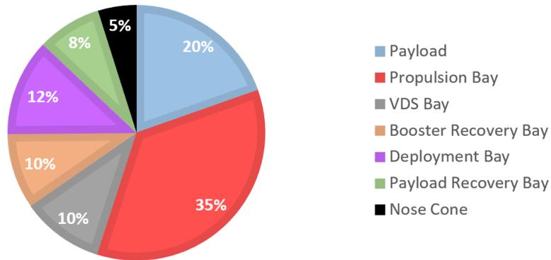
**Figure 82: Launch vehicle sub-system weight breakdown.**
