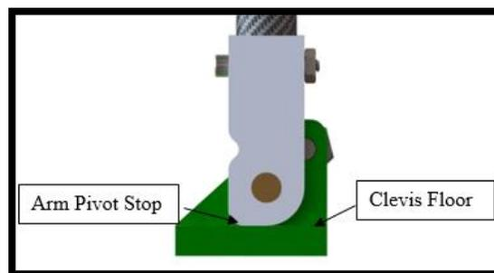
**Figure 113: Section view displaying Arm Pivot mechanical stop contour against Arm Clevis floor.**
