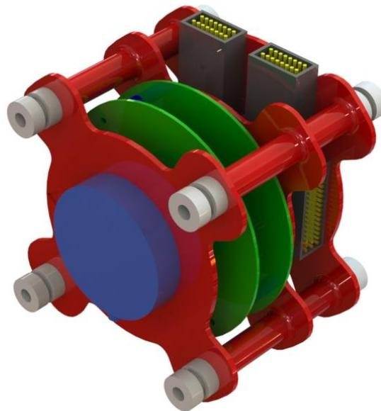
**Figure 130. Rendering of Flight and Redundant Recovery Electronics Assembly.**
