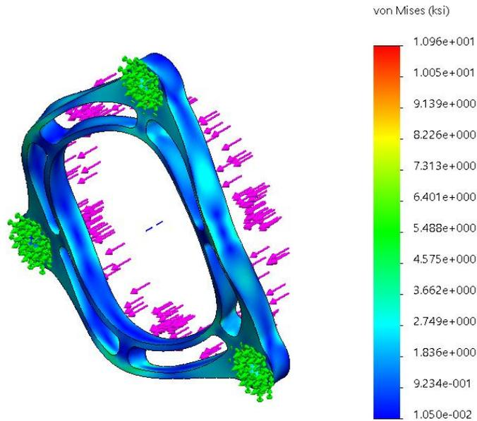
**Figure 34: Motor retainer FEA simulation stress plot.**
