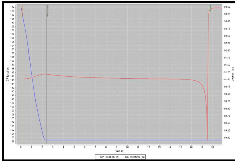
Figure 71: A plot of CG and CP locations versus time.
