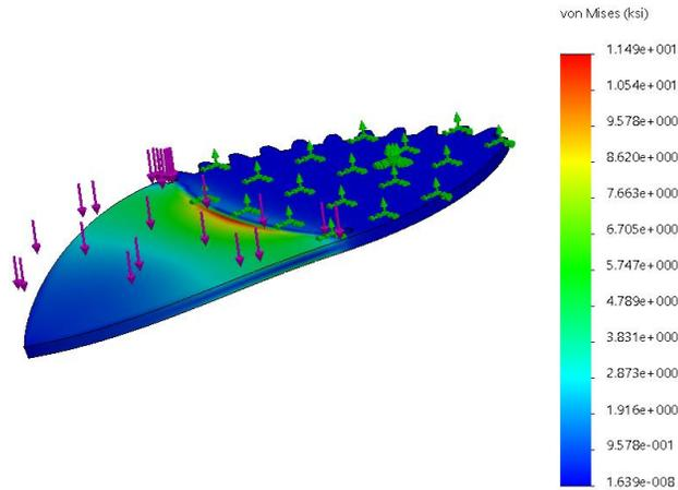
**Figure 22: Drag blade FEA stress plot.**
