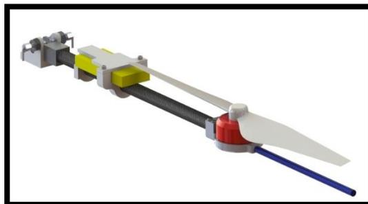
**Figure 109: Rendering of the Propulsion Arm in the deployed configuration.**
