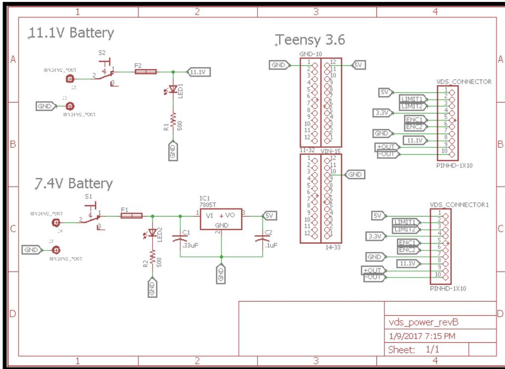
**Figure 7: Power distribution board revision B.**
