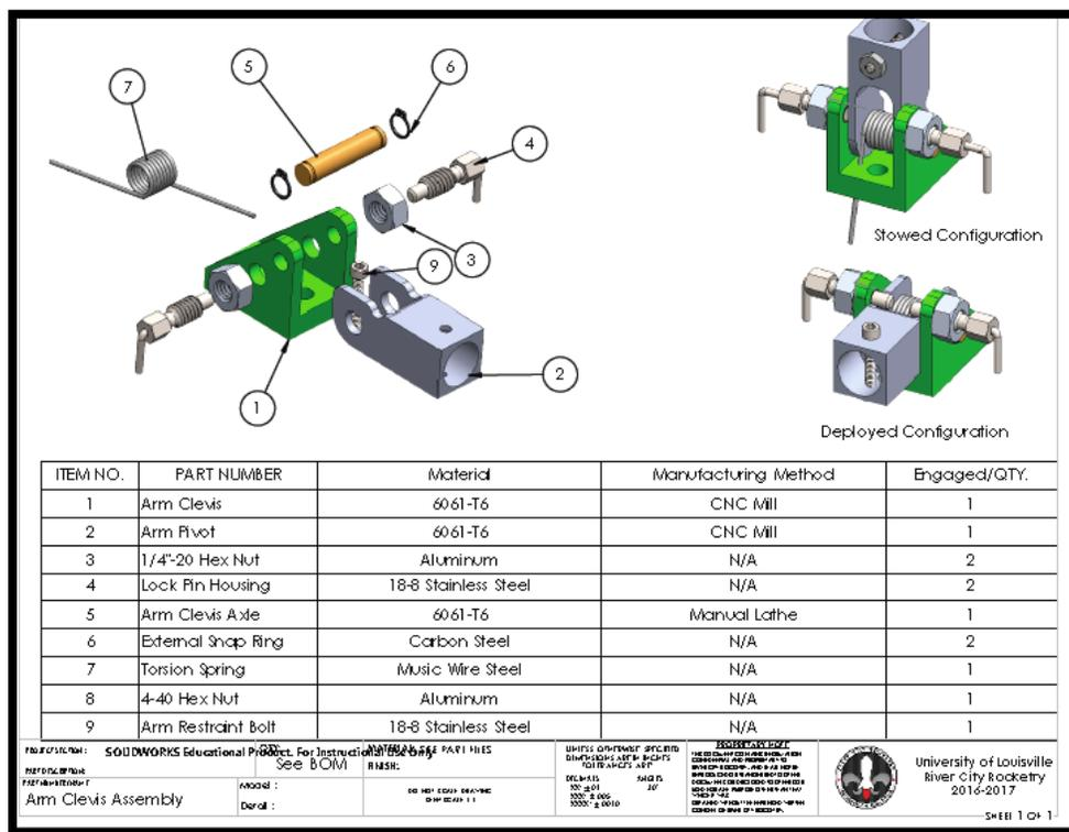
**Figure 110: Detailed drawing and exploded view of the Arm Pivot Assembly.**
