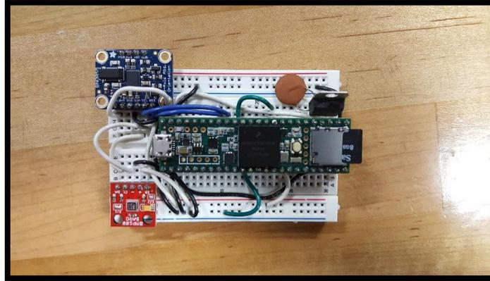
**Figure 46: VDS Test Electronics**
