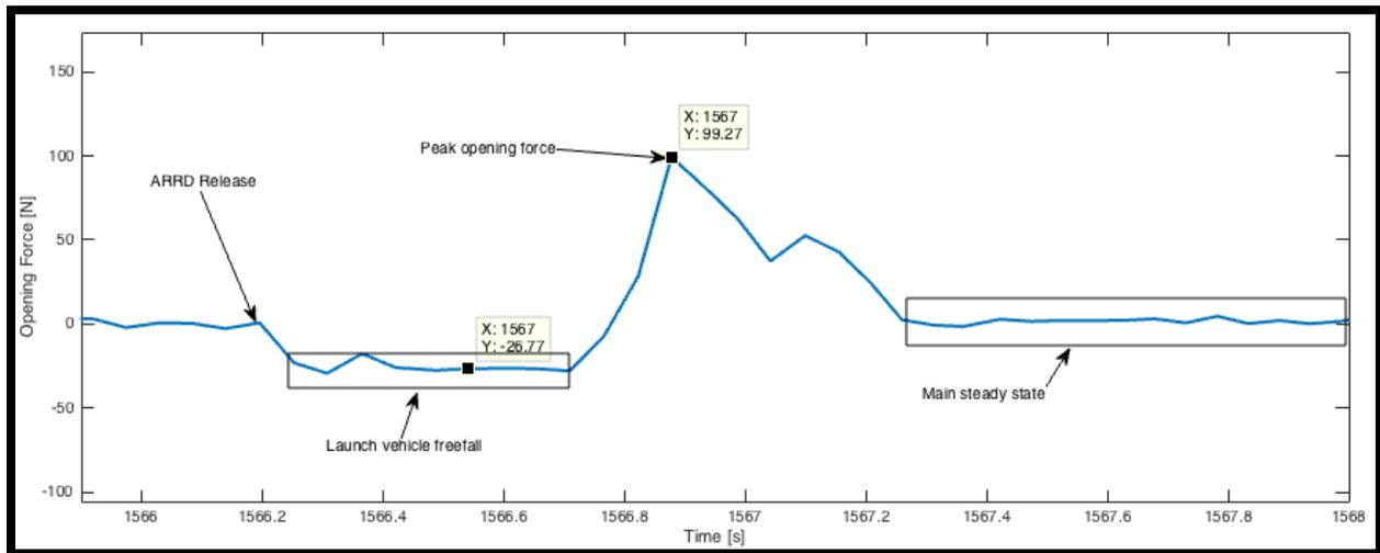
**Figure 54: Force curve during main opening.**
