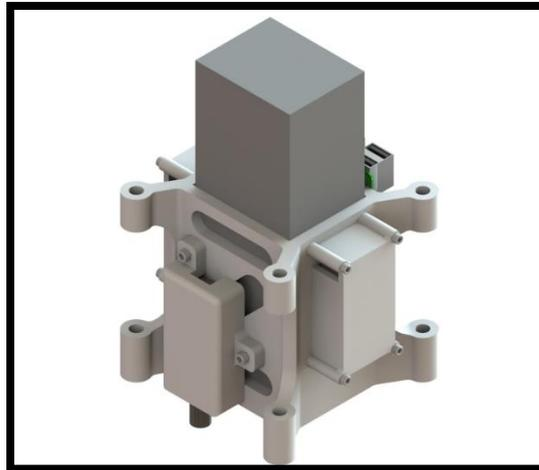
**Figure 132. Battery Module Rendering.**
