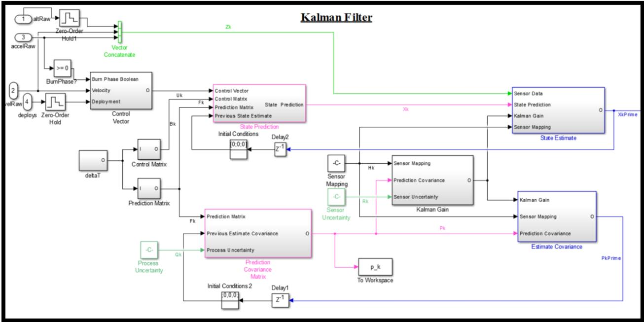
Figure 76: VDS simulation model of Kalman Filter.
