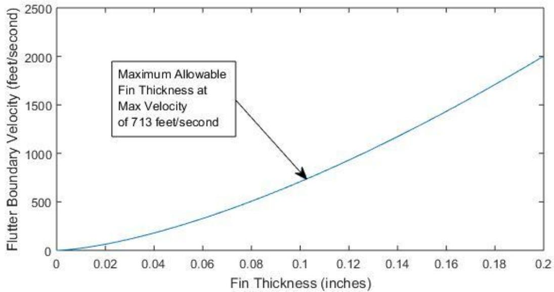
**Figure 80: Fin Flutter Velocity vs Fin Thickness**
