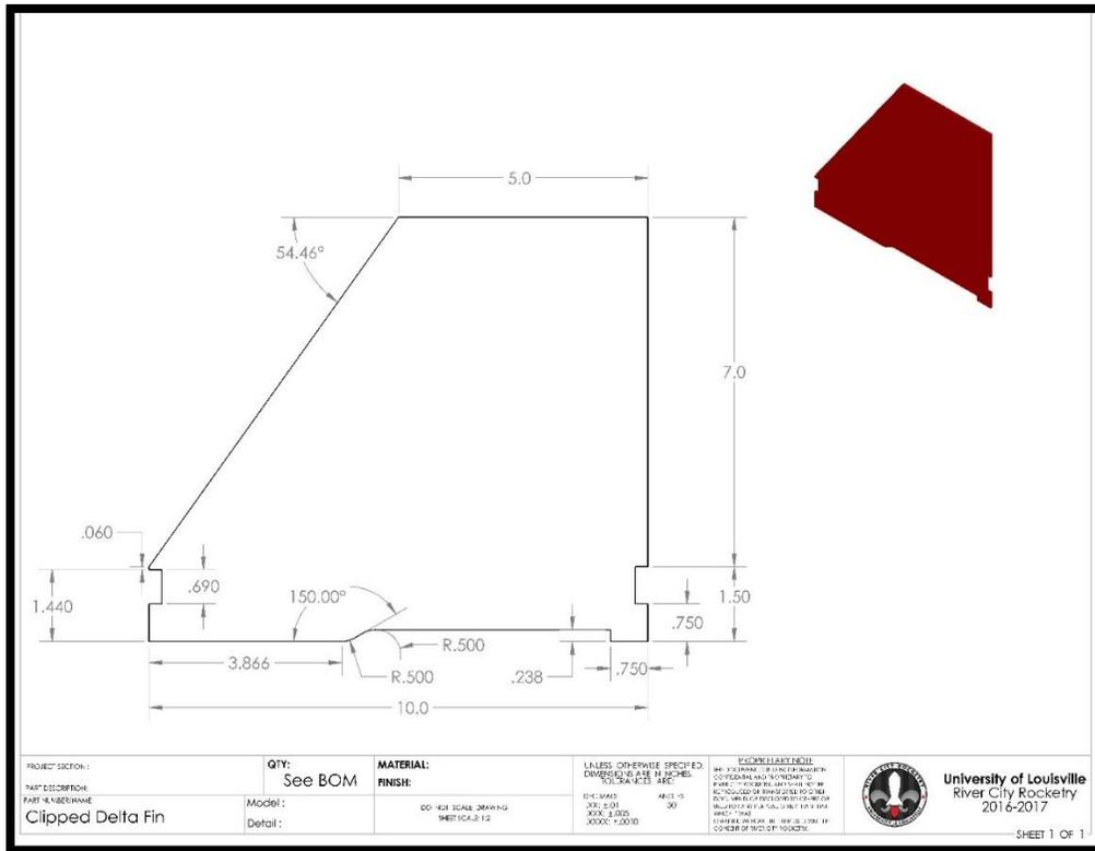
**Figure 35: Detailed drawing of fin shape.**
