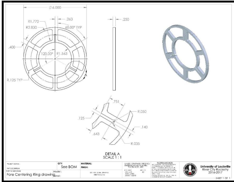
**Figure 30: Detailed drawing of fore centering ring**
