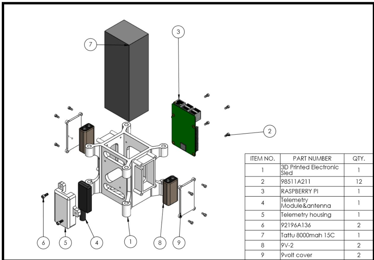
**Figure 133: Detailed drawing of the 3D Printed Batter Sled.**
