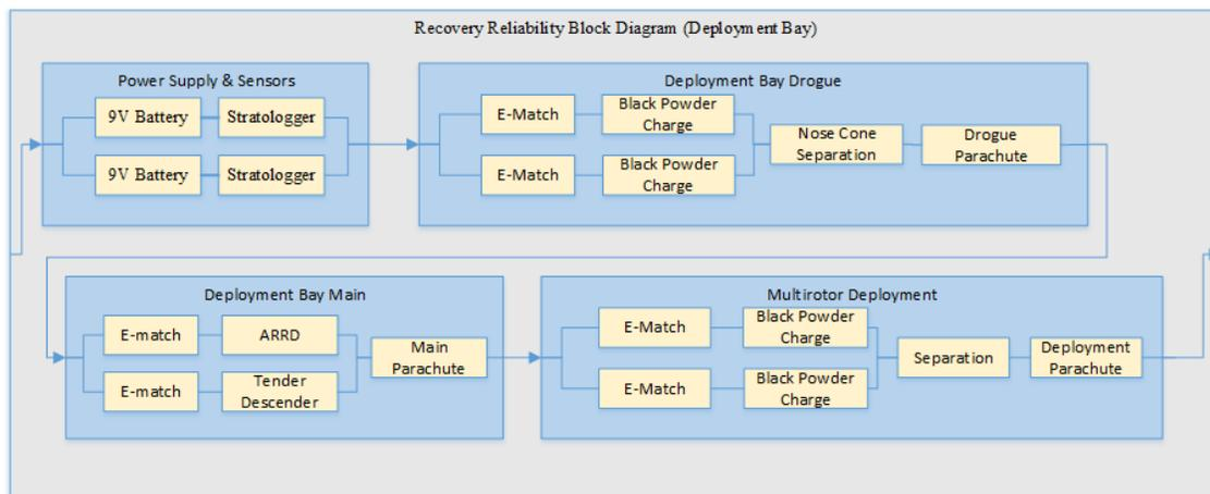
**Figure 90: Reliability block diagram for deployment bay.**
