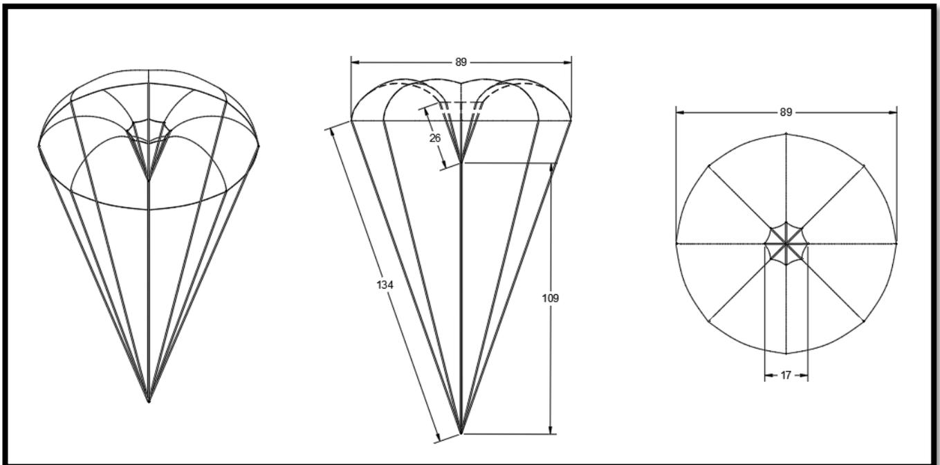
**Figure 63: Booster main parachute dimensions**
