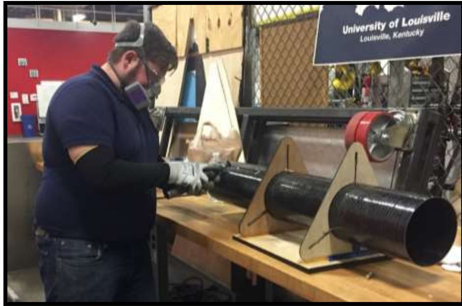
Figure 57: Cutting of the fin slots in the booster airframe.
