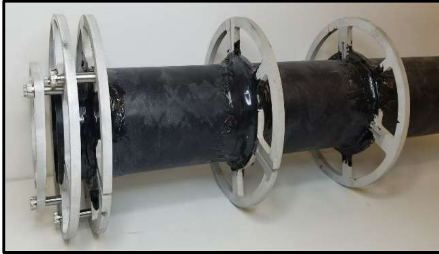
Figure 54: Centering rings epoxied onto the motor mount tube.
