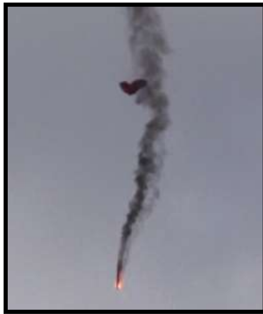
Figure 114: Booster section in freefall after the shock chord burned.
