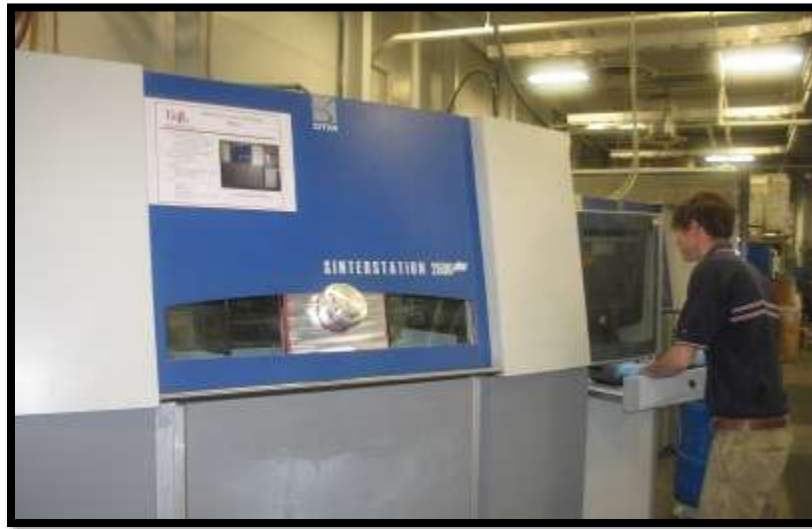
Figure 65: SinterStation 2500+ machine used to additively manufacture the nose cone.
