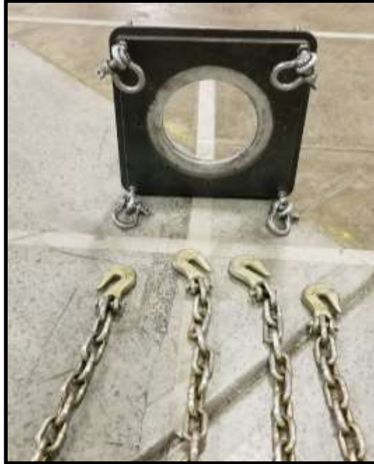
Figure 38: Plates and chains used to push the airframe off of the mandrel.
