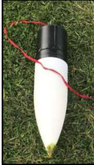
Figure 66: Additively manufactured parabolic nose cone following successful drop dest.
