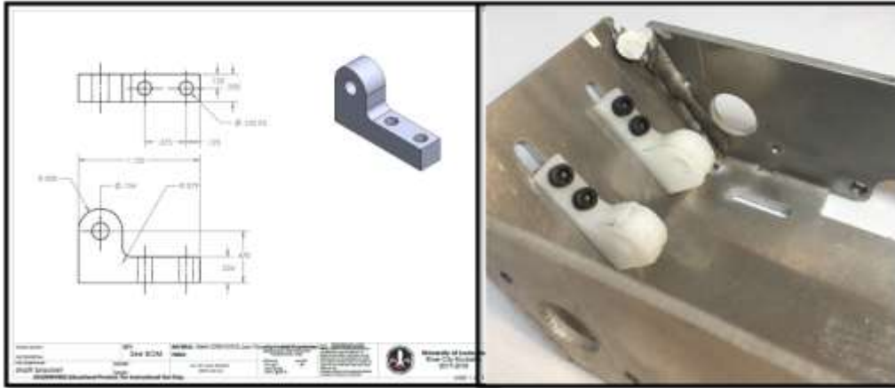
Figure 174: Drive shaft spacer drawing and manufactured drive shaft spacer.
