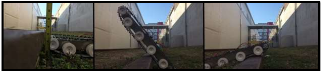
Figure 177: 3.25 inch vertical step.
