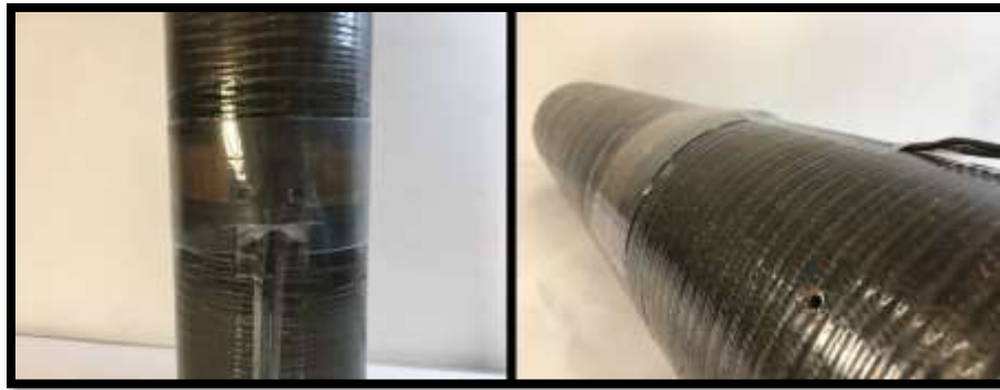
Figure 157: Receiver antenna adhered to airframe.
