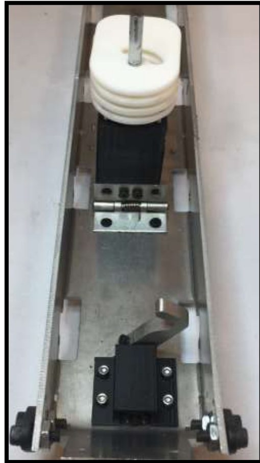
Figure 202: Top view of the tow assembly before and after locking motor rotation.
