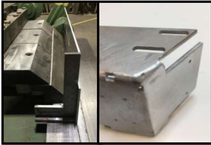
Figure 162: Rover body bending and welded seam.
