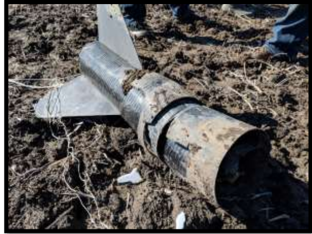
Figure 120: Damage to the booster section.
