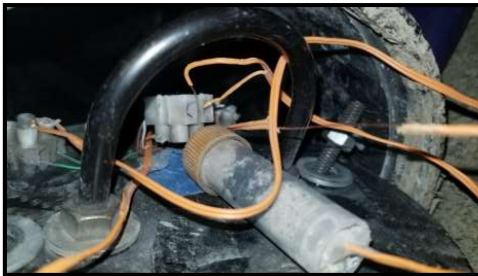
Figure 121: Unignited redundant ejection charge.
