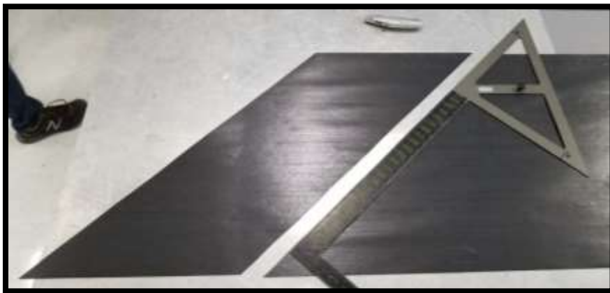
Figure 39: Fin material being cut.
