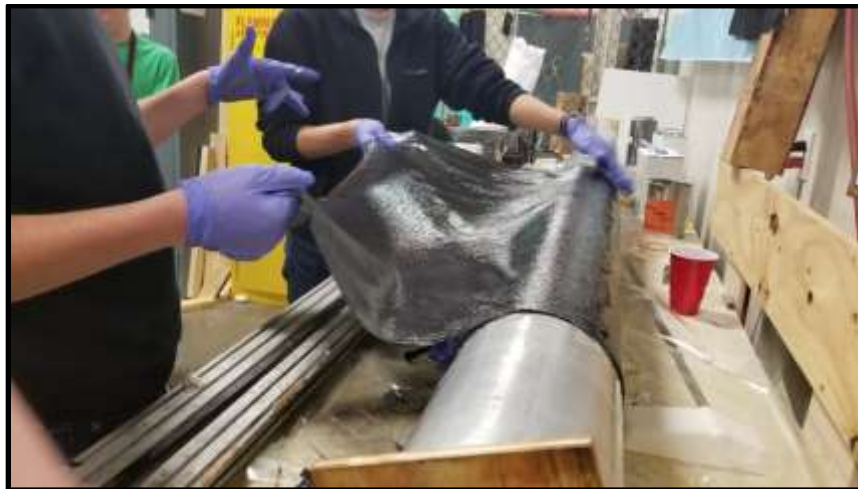
Figure 33: Lay-up of individual carbon fiber sheets onto aluminum mandrel.
