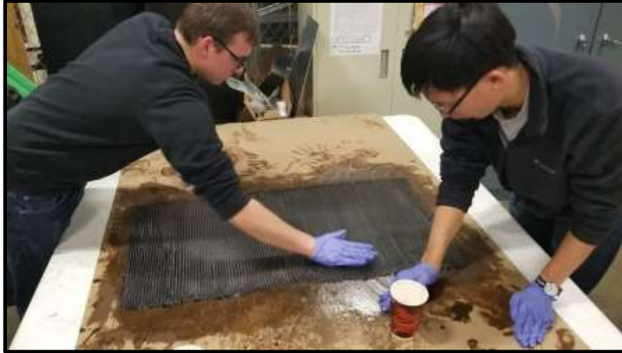
Figure 32: Saturation of quasi-isotropic carbon fiber sheets with epoxy.
