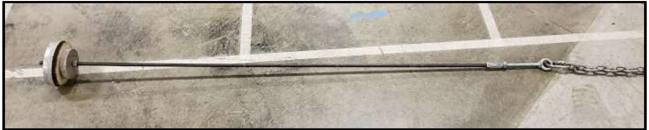
Figure 36: Threaded rod and attached components used during airframe removal process.
