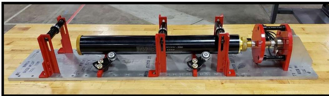
**Figure 41: Solid motor test stand with 75mm motor.**
