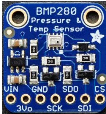
**Figure 29: Adafruit BMP280 – Barometric Pressure and Temperature Sensor**
