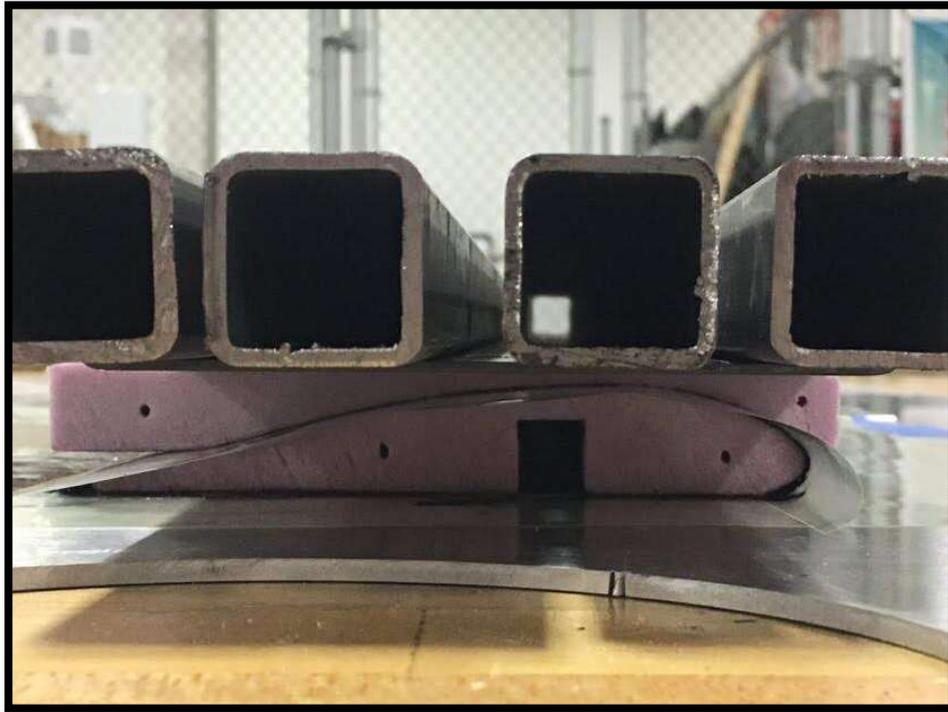
**Figure 89: Carbon fiber wing curing under weight.**
