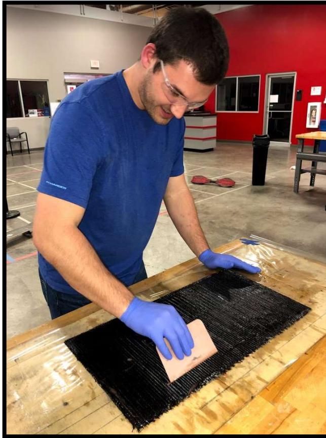
**Figure 87: Wing carbon fiber layup.**
