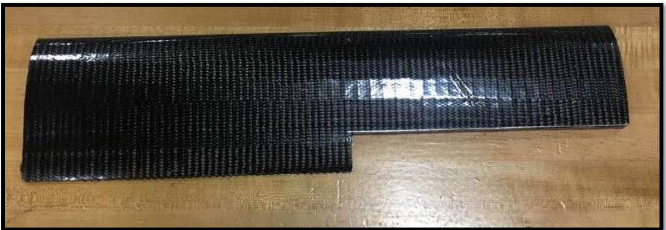
**Figure 90: Carbon fiber wing without wooden supports and control surfaces.**
