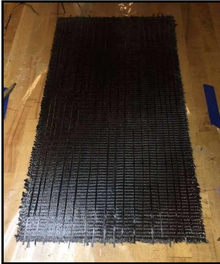
**Figure 88: Carbon fiber filaments layed on carbon fiber sheet.**
