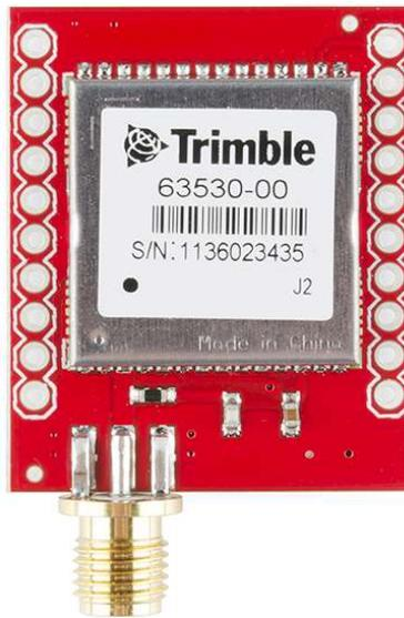
**Figure 31: SparkFun Copernicus II Breakout (12-Channel)**
