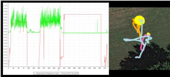
Compass noise vs. thrust (left), Oscillation around a central point (right)
