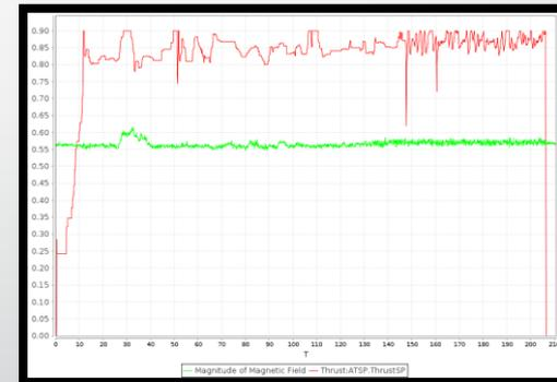
Noise eliminated after GPS/Compass module moved
