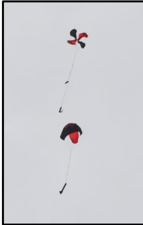
Figure 3: Custom vortex ring and cruciform parachute safely recovering rocket at competition.
