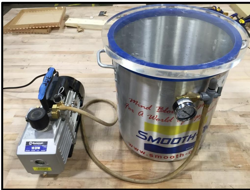
Figure 72: Vacuum chamber and pump used for StratolLogger tests.
