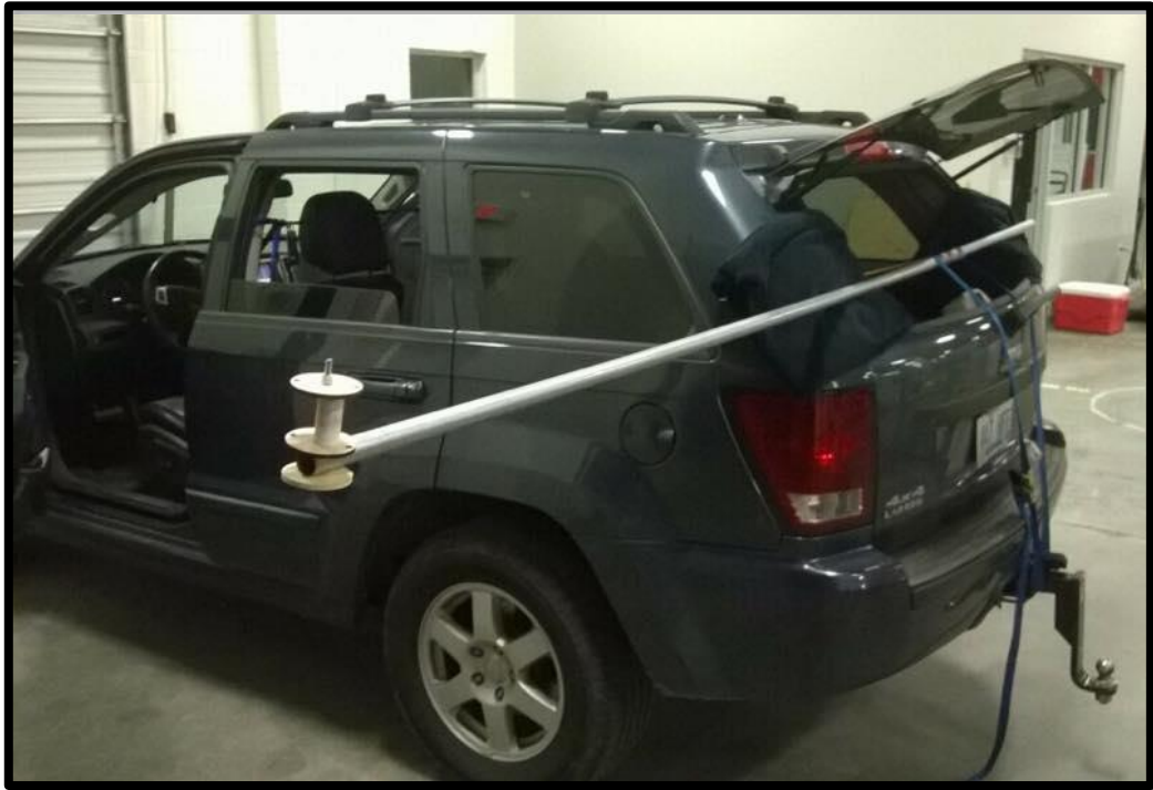
Figure 190: Subscale parachute testing rig.
