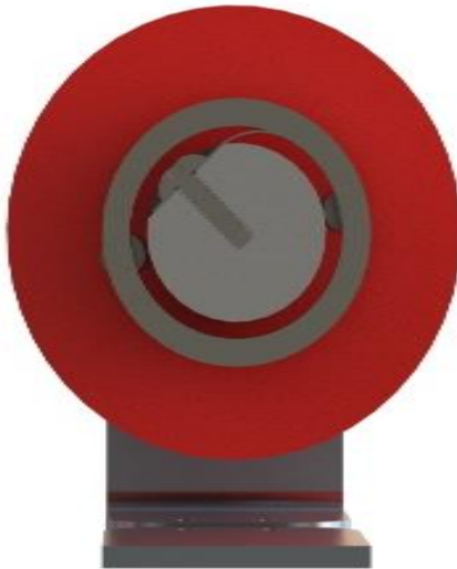
Figure 146: Cross section view of the constant force spring on shaft.
