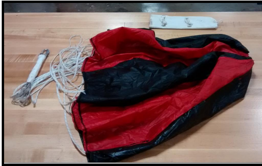
Figure 59: Parachute and deployment bag laid out.
