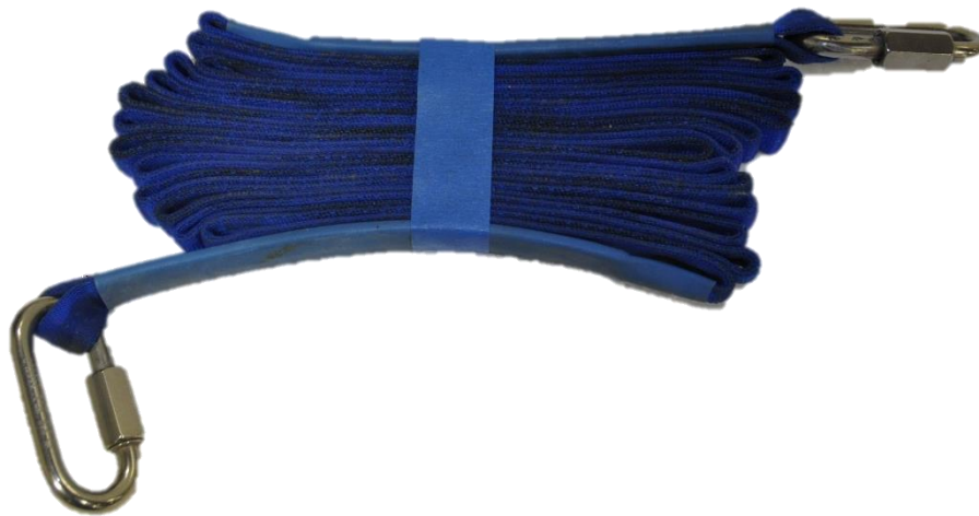
Figure 58: Shock cord folding method.
