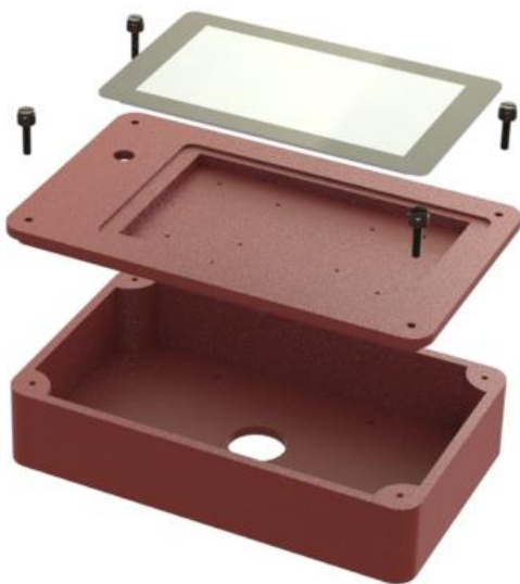
Figure 88: Exploded view of HMI enclosure.
