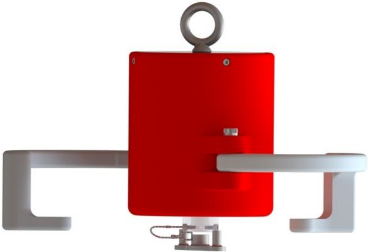
Figure 49: Master link black powder charge container in de-reefed state.
